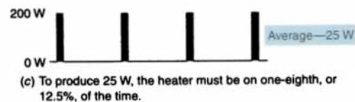
FIGURE 14-15 Time proportioning of a 200 W heater element.
