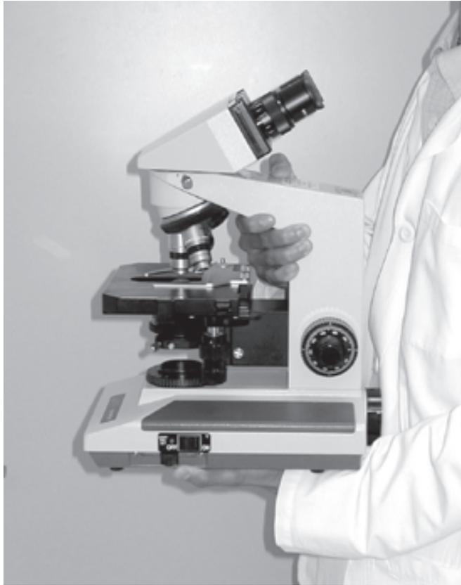
The condenser can be lowered or raised by an adjustment knob. Lowering the condenser decreases the amount of light that reaches the object. This is usually a disadvantage in microbiological work. It is best to keep the condenser fully raised and to adjust light intensity with the iris diaphragm.
