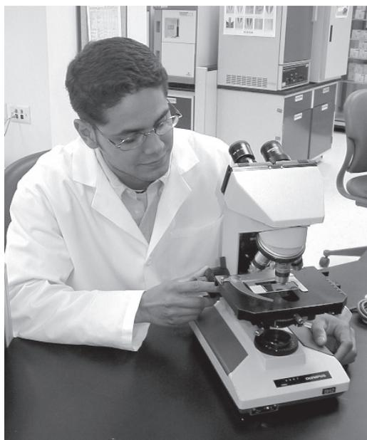
Turn the adjustment knobs *slowly* and *gently*, as you pay attention to the relative positions of the objective and object. Avoid bringing the objective *down* with the fine adjustment while viewing, because even this slight motion may force the lens against the object. Bring the lens safely down first with the coarse knob; then, while looking through the ocular, turn the fine knob to *raise* the lens until you have a clear view of the subject.
