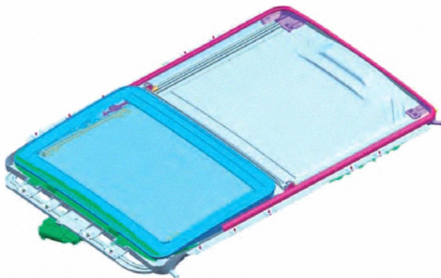
Figure 9.6.1 Sunroof of the BMW 7 Series (courtesy of BMW).
