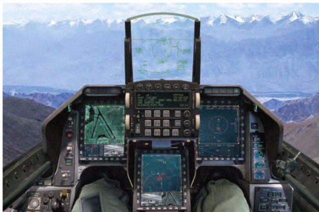
Figure 7.11.1 F-16 cockpit and avionics system controls (courtesy of Lockheed Martin).
