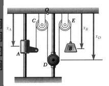
• Pulley *D* has uniform rectilinear motion. Calculate change of position at time *t*.
