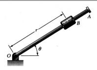
Rotation of the arm about O is defined by  $\theta = 0.15t^2$  where  $\theta$  is in radians and t in seconds. Collar B slides along the arm such that  $r = 0.9 - 0.12t^2$  where r is in meters.
