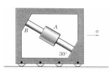
The collar A is free to slide along the smooth shaft B mounted in the frame. The plane of the frame is vertical. Determine the horizontal acceleration *a* of the frame necessary to maintain the collar in a fixed position on the shaft.
