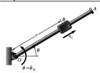
A block *B* of mass *m* can slide freely on a frictionless arm *OA* which rotates in a horizontal plane at a constant rate  $\dot{\theta}_0$ .
