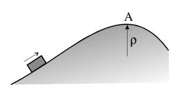
Determine the maximum speed, v, which the sliding block may have as it passes point A without losing contact with the surface
