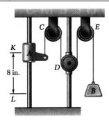
Pulley D is attached to a collar which is pulled down at 3 in./s. At t = 0, collar A starts moving down from K with constant acceleration and zero initial velocity. Knowing that velocity of collar A is 12 in./s as it passes L, determine the change in elevation, velocity, and acceleration of block B when block A is at L.
