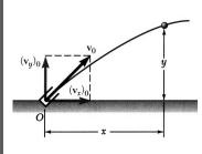
• Rectangular components particularly effective when component accelerations can be integrated independently, e.g., motion of a projectile,
