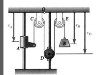
• Differentiate motion relation twice to develop equations for velocity and acceleration of block *B*.
