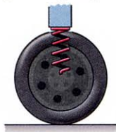
Simplified spring detail
