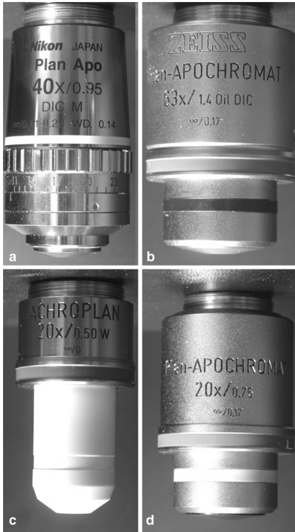
Fig. 3.4 Various types of objective lenses showing inscriptions on the barrel of the objective. (a) \times 40 Plan Apo with correction collar for adjustment to correct for coverglass thickness and refractive index mismatch; (b) \times 63 Plan Apo oil immersion; (c) \times 20 Plan Achromat water immersion; (d) \times 20 Plan Apo
