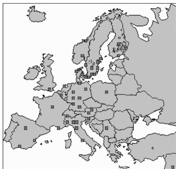
FIG. 1—Distribution of buildings in Europe, where bowing or distortion of the marble cladding has been recorded by the TEAM partners.
