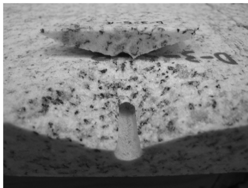
FIG. 8—Spall from edge dowel test.
