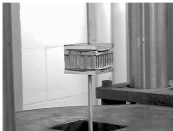
FIG. 2— Modified ASTM D897-tensile bond test.
