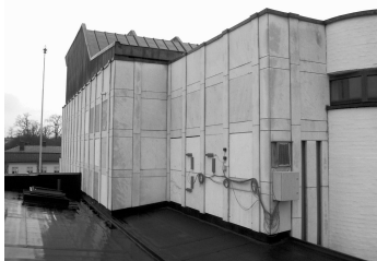
FIG. 4—Test site at the city hall of Nyköping. Different marble, different thickness, and chemical treatments are tested together with monitoring of temperature and strain.
