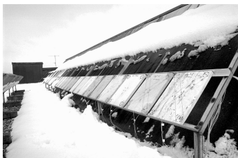
FIG. 11—Field exposure site in Ljubljana, Slovenia. Sample sizes are 30 by 400 by 500 mm.
