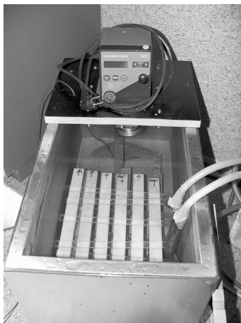
FIG. 10—Laboratory test for moisture and heat-induced expansion, providing relevant data for dimensioning of dilatation joints. Sample sizes are 30 by 30 by 200 mm.
