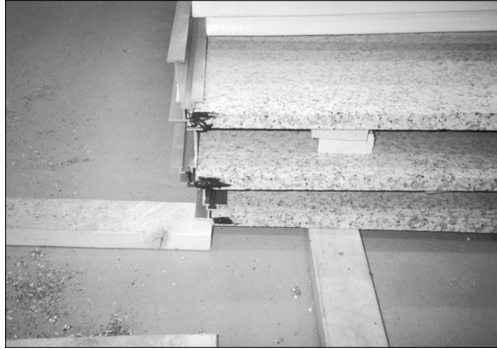
FIG. 5—Edge view of full-width kerf anchors.
