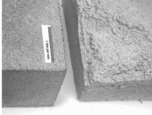
FIG. 25—Photomicrograph of Indiana Limestone from two different locations shown after accelerated weathering.
