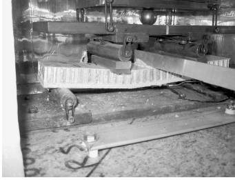
FIG. 1— ASTM C880-flexural strength test.
