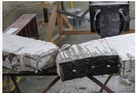
b) Hinging and fracture, Bm-Col 2
