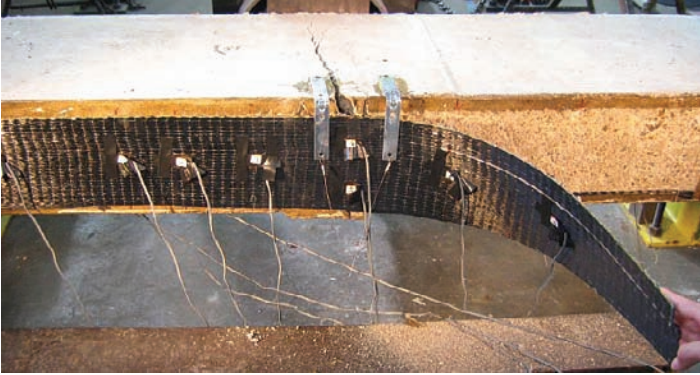
Fig. 7 Delamination failure of Beam 1
