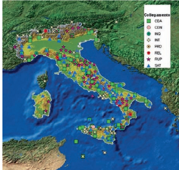
Fig. 9 Italian INGV seismometric network (See also Color Plate 8 on page 212)
