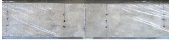
b) Separation using clear polyethylene wrap, Beams 4 and 5
