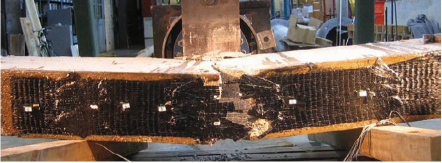
Plate 2 Fracture of CFRP sheet in Beam 2 (See also Fig. 8 on page 27)
