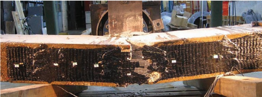
Fig. 8 Fracture of CFRP sheet in Beam 2 (See also Color Plate 2 on page 210)
