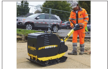
Vibrating plate compactor
