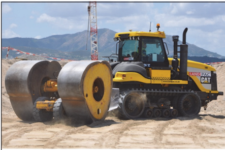
High energy impact compaction (HEIC) roller
