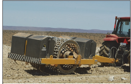
Towed grid roller
