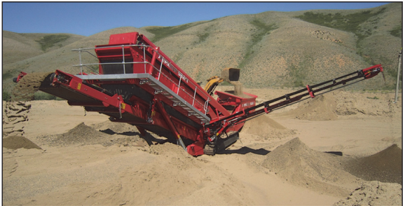
Mobile vibrating screen for use with sand and gravel (shown here separating fines from a granular fill)
