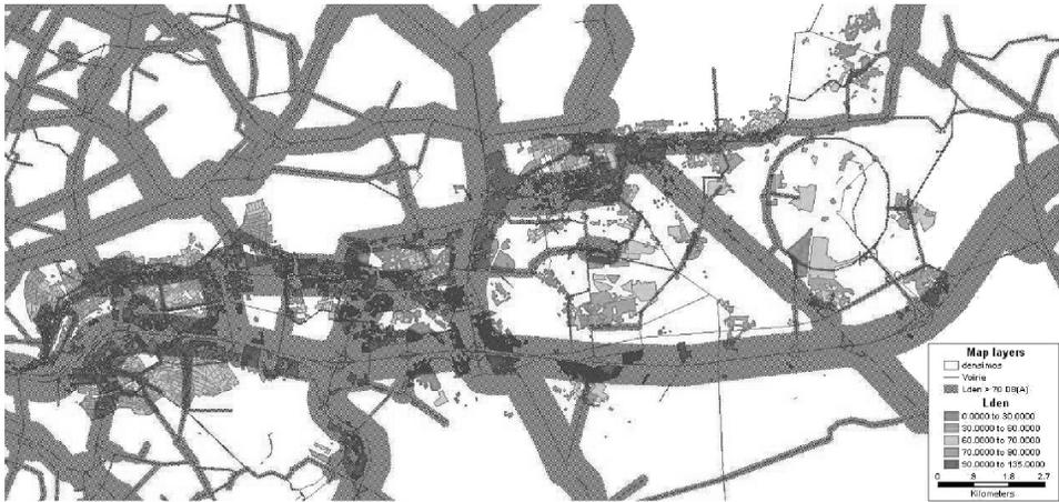
Figure 15.6 Strip exposed to 70+ dB in Marne la Vallée during morning rush hour, 2008.
