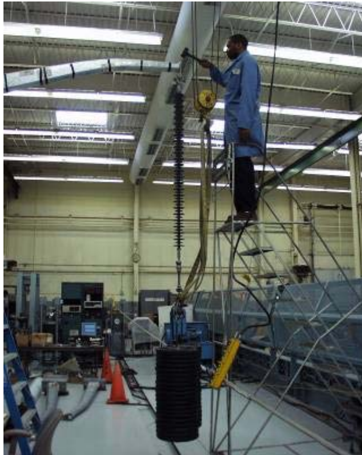
Figure 11 – Fundamental Frequency Test Setup
