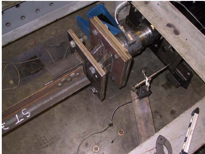
Figure 2, Single Leg Bolted at Both Ends, Type 2
