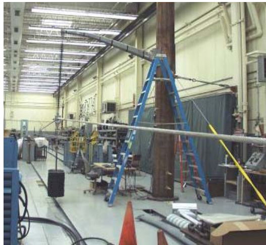
Figure 13 – Span Test Setup
