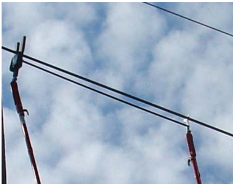
Figure 6 - Sensorlink's Ohmstik modified to make resistance readings over five feet instead of one foot to increase the accuracy of the instrument.
