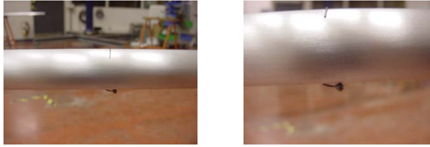
Figure 3: Details showing installation of the corona calibrating spheres
