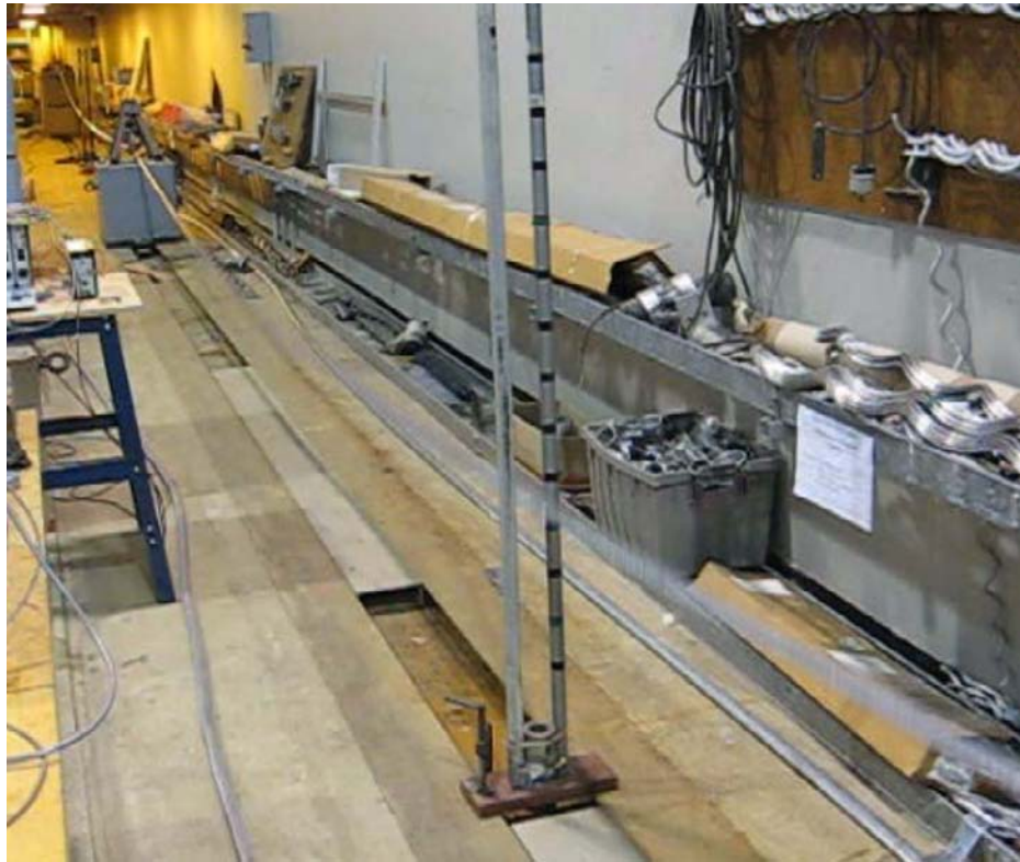
Figure 3 – Setup for Galloping Conductor Test
