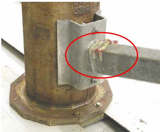
Figure 6 – Strain Gauge Placement
