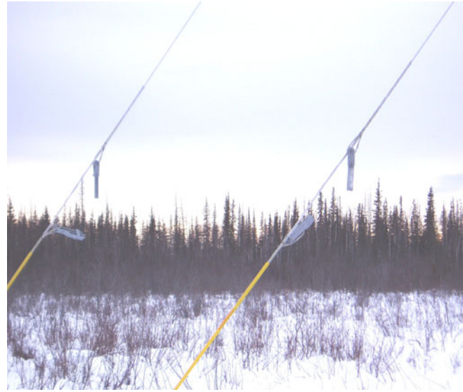
Fig. 8a (left) X-tower with shear release mechanism
