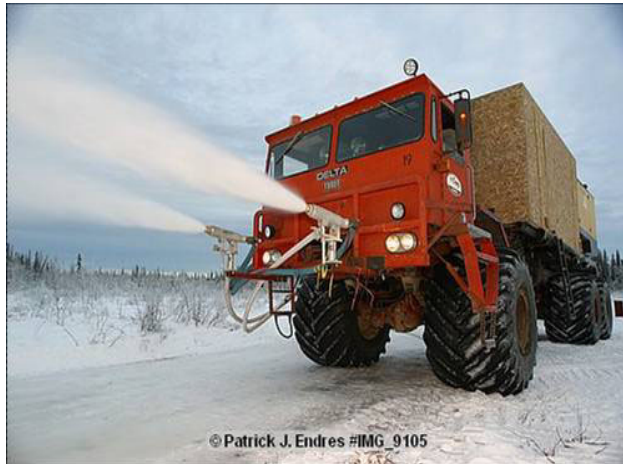
Fig. 11a (above left) Truck with water tanks and snow guns (Used with Permission)
