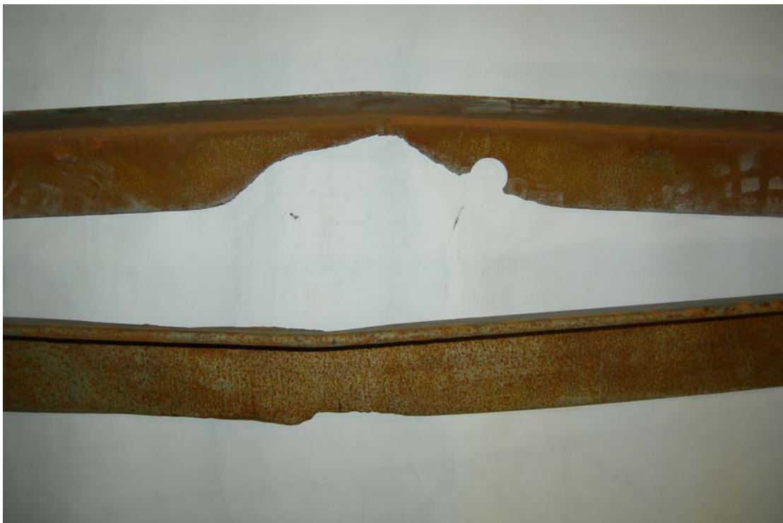
Figure 7 Perforated members 95L-40-2 and 48L-40-2.
