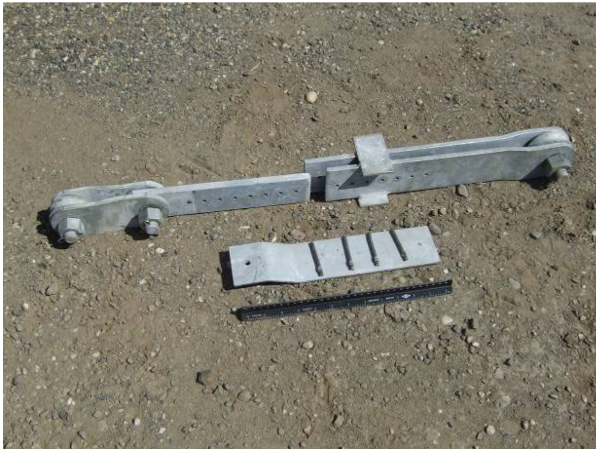
Fig. 7 Guy strand shear release mechanism
