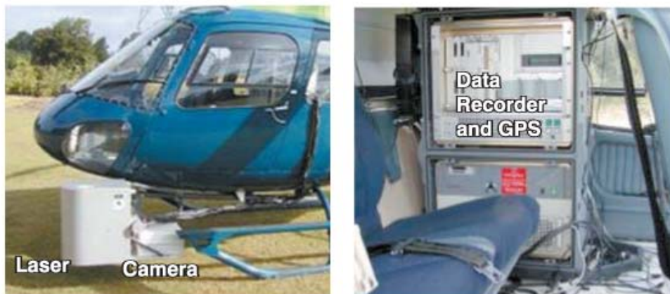
Figure.6: Optech Incorporated's ALTM 2050 airborne laser scanner. The laser is attached to the front of a Squirrel helicopter with a purpose built mount. The metric camera is installed just behind the scanner, and both of these sensors feed data to the recorder contained within the aircraft.
