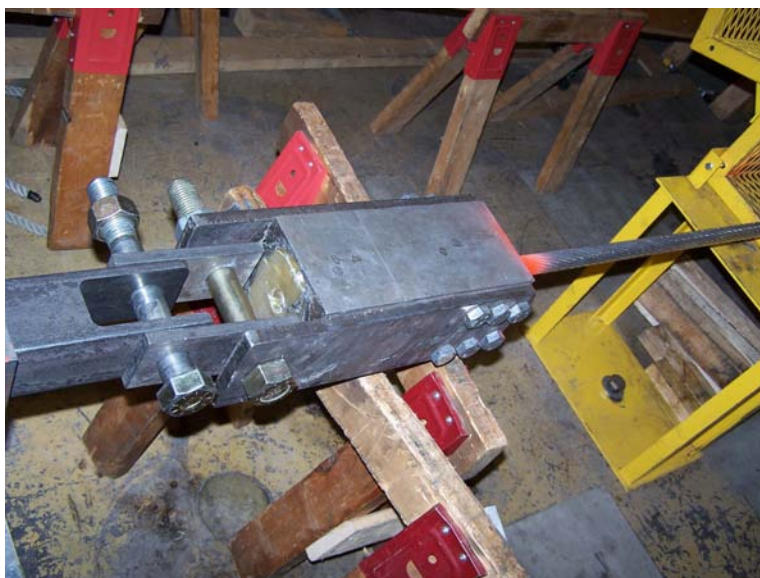
Figure 7 – Poured Epoxy Deadend
