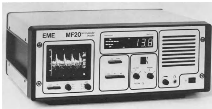
Fig. 1. Microvascular Doppler system with built-in real time spectrum analyzer
