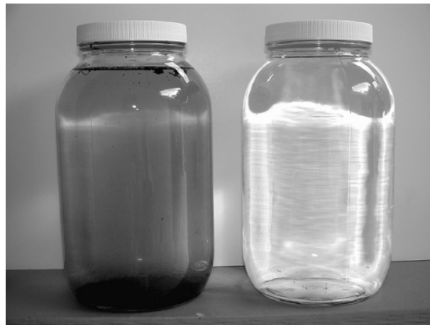
FIGURE 7-1 (Left) Sample of storm water runoff collected from Helotes Creek in the recharge zone of Comal Springs, Edwards Aquifer, Texas. (Right) Sample taken from Comal Springs on the same day; the springs are known for their clarity. (Photograph courtesy of Gregg Eckhardt.)
