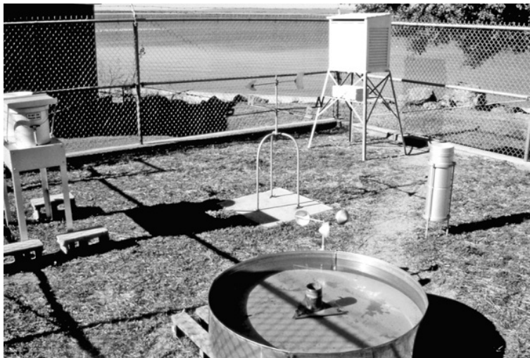
FIGURE 5-21 Hydrometeorologic station equipped with instruments for measurements of direct evaporation (pan evapometer in the front), wind speed, precipitation, air temperature, and insolation (hours of sunshine).
