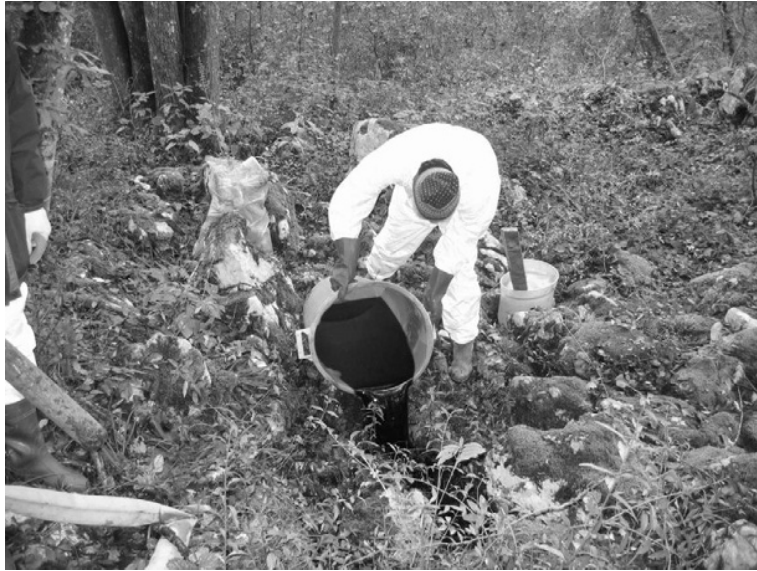
FIGURE 3-9 Injection of an uranine solution into a fissure at the margin of the landfill. (Photo: Petrič, 2005.)
