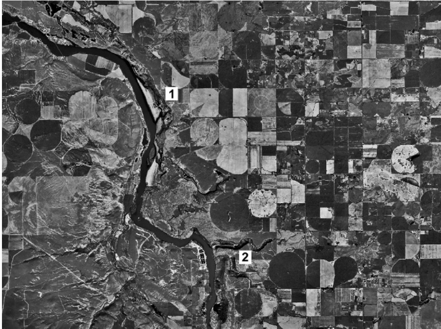
FIGURE 1–20 Intensive center-pivot irrigation using groundwater from the same aquifer supplying water to numerous springs along the right bank of the Snake River, Idaho: (1) Thousands Springs area; (2) Box Canyon Springs, also shown in Figure 1–16 . (Photograph courtesy of USGS.)
