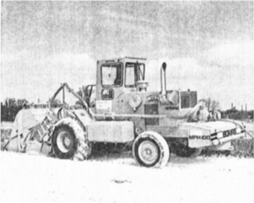
Figure 10.2 Autograder producing mix-in-place stabilized soil (courtesy Bomag Ltd) (Figure 10.4(a)). Increased pulverization increases the strength of soil-cement. Ideally the degree of pulverization, if the larger stone particles are excluded, should break down to parent soil so that 80% of the particles are less than 5 mm and mixing should be uniform. A lengthy period of mixing brings about partial hydration of the cement with a resultant loss of strength at constant density. If compaction is delayed the cement begins to hydrate and therefore the soil-cement begins to harden. As a result the mixture becomes more difficult to compact. Compaction should be completed within two hours of mixing. The strength of soil-cement gradually increases as the time taken in curing increases (Figure 10.4(b)). Also, the higher the temperature, the more rapid is the gain of strength. Soil-cement will harden in cold weather providing the temperature does not fall below 0°C. Excessive drying increases strength but tends to crack the soil-cement. By contrast, strength is reduced by soaking (Figure 10.5). This is particularly the case with clayey soils. Typical ranges of 7- and 28-day unconfined compressive strengths for soaked soil-cement specimens are given in Table 10.3. It is recommended by Anon. (1990(d)) that specimens are soaked before being tested since soil-cement may become intermittently or permanently saturated during its service life and it possesses lower strength under saturated conditions.
