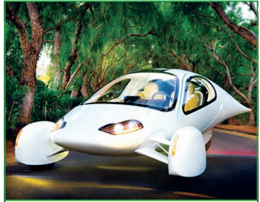
Automakers produce concept cars to test innovations in fuel use, aerodynamics, materials, and design. These models are not ready for highway use, but the innovations they possess might become part of cars in the future. The car pictured here is the Aptera made by Aptera Motors, Inc. This model is completely electric. The company has also developed an electric/diesel hybrid Aptera, which gets 330 miles per gallon (140 km/l). (Aptera Motors, Inc.)
