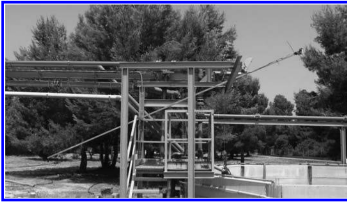
Figure 3. Camera placed on top of the tank for velocity measurements.
