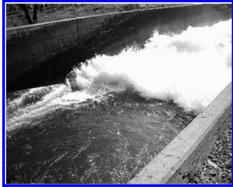
Figure 4. Detail of the turbulence due to the bottom step.
