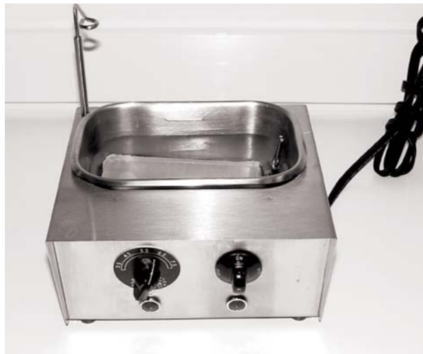
FIGURE 4.2: A thermostatically controlled water bath. This water bath maintains a steady softening temperature and is ideal for softening impression compound
