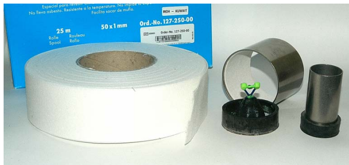
FIGURE 18.1: A roll of ring liner, a rubber crucible former with attached wax pattern and casting rings
