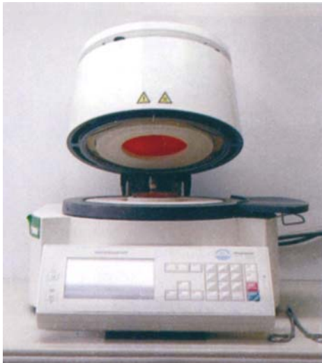
FIGURE 20.4E: After each application the porcelain is fired in a computer controlled porcelain furnace at high temperatures
