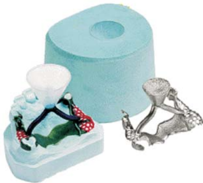
FIGURE 16.3A: An assembled RPD pattern (lower left) made from ready made casting waxes on a refractory cast. The sprue formers have been attached. The pattern is invested in a suitable refractory material to create a mold (behind). The completed casting is shown on the right side
