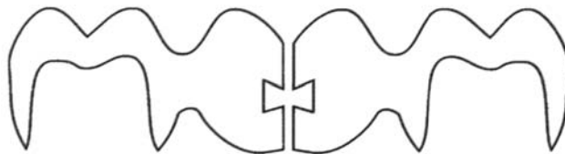
FIGURE 22.4: A mechanical interlocking design between two parts to be joined by cast-metal
