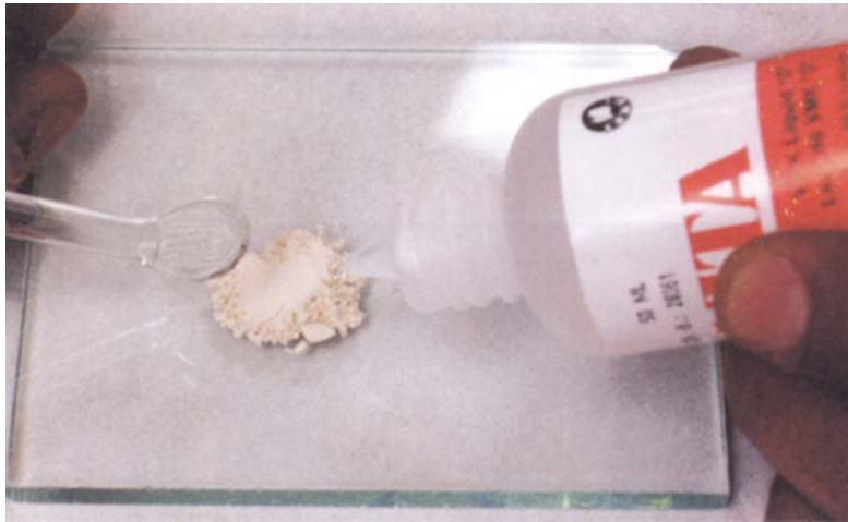
FIGURE 20.4A: Opaquers powder is a dense cream colored powder used to hide the metal. It is mixed with the modeling liquid to produce a sandy mix. A glass spatula is used for mixing as metal might abrade and contaminate the porcelain
