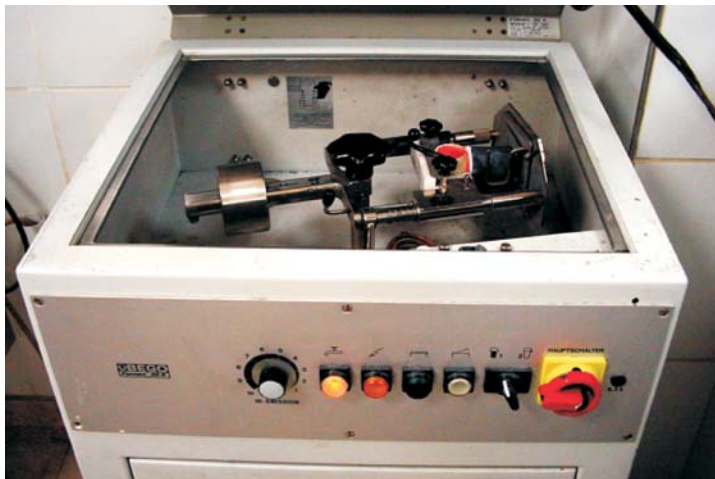
FIGURE 18.6: An induction casting machine. The molten metal is driven into the mould by centrifugal force. One arm of the machine has a counter weight which balances the weight of the arm carrying the crucible and mould as it rotates. The red hot crucible and the casting ring is visible in the machine. The induction coil (copper colored) is half visible and is used to melt the metal
