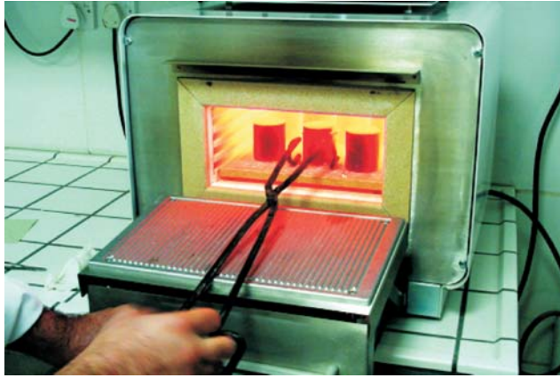
FIGURE 18.4: The burnout furnace. The wax pattern is vaporized in this furnace leaving behind an empty mould space. The furnace also increases the size of the mould (thermal expansion) which helps to compensate for casting shrinkage
