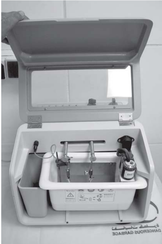
Figure 23.2: An electrolytic polishing unit. The casting is suspended inside the bath (anode). Polishing is achieved when minute quantities of oxide and surface metal is removed electro-chemically
