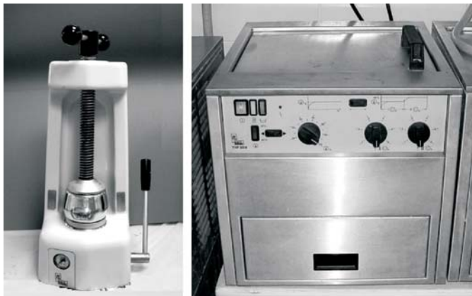
FIGURE 8.6: Left—A hydraulic press (Kavo) is useful for trial and final closure of the flask. The pressure indicator dial indicates the pressure that is applied. Right—An automated curing bath (Kavo). The time and temperature of the curing cycle can be preset and regulated for optimum cure
