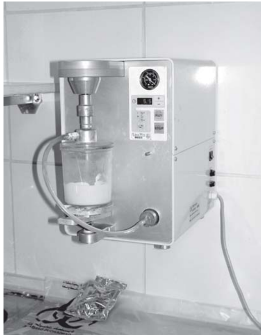
FIGURE 18.3: An investment mixer (Bego - Germany). The investment is mixed under partial vacuum in order to minimize voids in the mix
