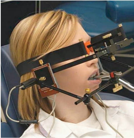
Fig. 14.6 A kinematic facebow in use. Two styli are attached to the mandible and two sensor pads are fixed to the head alongside the area of the temporomandibular joints.
