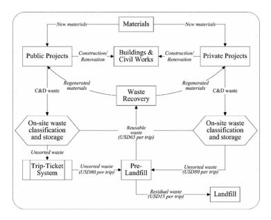
Figure 5.4 A simple TTS-based simulation model.
