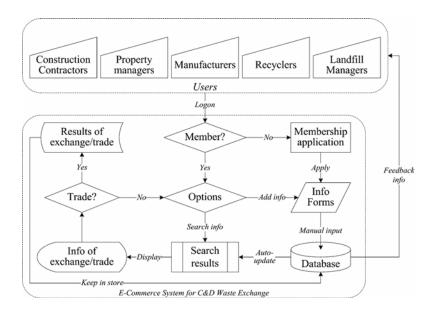
Figure 5.3 Webfill e-commerce model for C&D waste exchange.
