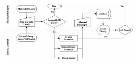
Figure 4.2 Data flowchart of the bar-coding system for group-based IRP.
