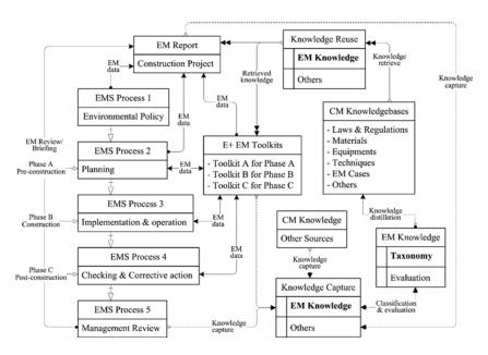
Figure 6.1 The prototype of the E+ model.
