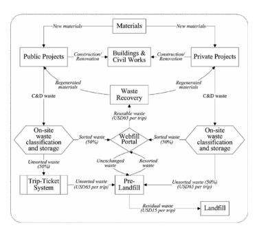
Figure 5.5 A proposed Webfill-enhanced TTS simulation model.
