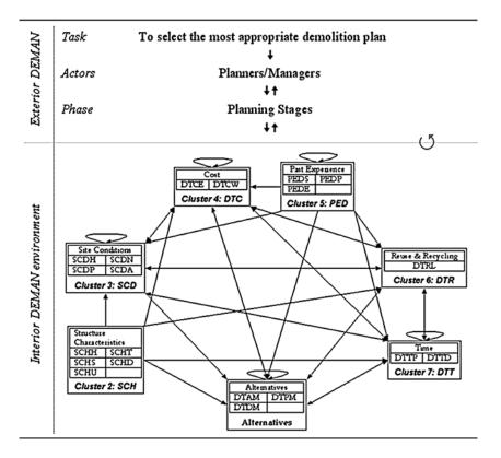
Figure 3.11 The ANP environment for demolition plan selection.
