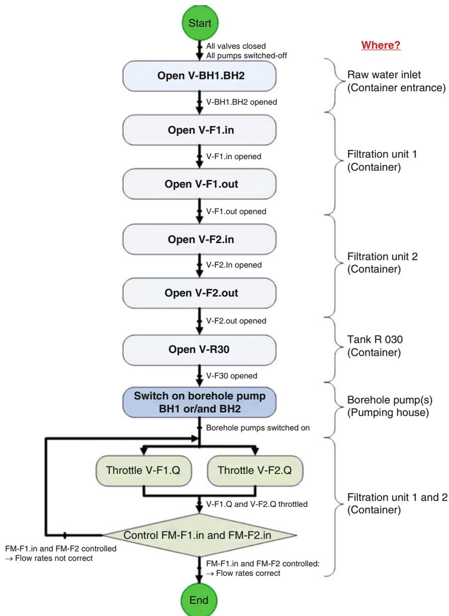
Picture 16: Operating instruction n° 1 – Starting the filtration unit
