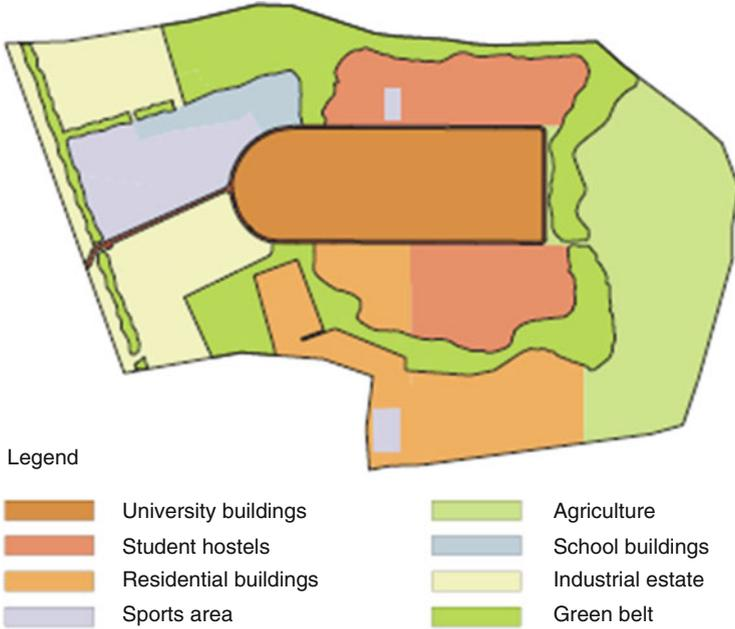
Fig. 4.49 VVU masterplan – partial concept: zoning of utilization
