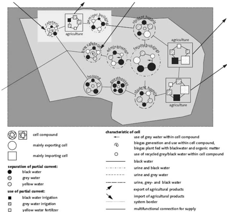
Fig. 4.46 Cell model for water cycling
