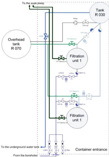
Picture 9: Schematic representation of the groundwater treatment plant (top view)
