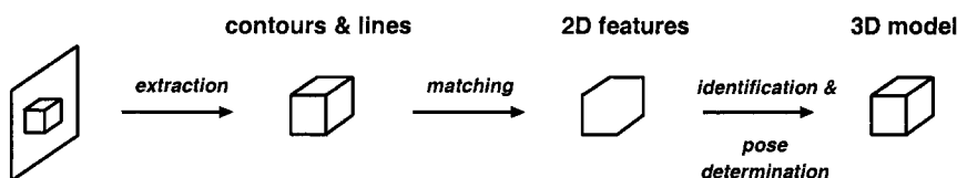
Figure 6: Roberts identification and pose determination system. The object was represented as a set of 3D coordinates representing the corners of a building block. Recognition evolved firstly by extracting contours and lines, followed by a matching process with stored 2D features, followed by eventual matching some of the possible models against the image.
