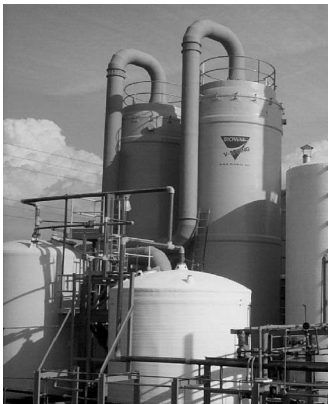
Fig. 16.4. Bioreactors treating \text{CS}_2 from waste gas at a fungicide manufacturing plant
