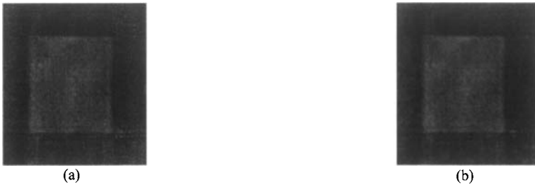
Figure 3. Example of use of median filtering: a)-PA-UT c-scan of panel B3 as inspected and b) PA-UT c-scan after 5x median filtering.
