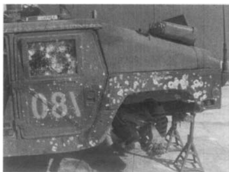
Figure 1: Attack by a small IED shows multiple impacts on the window indicating close proximity and high impact velocity.
