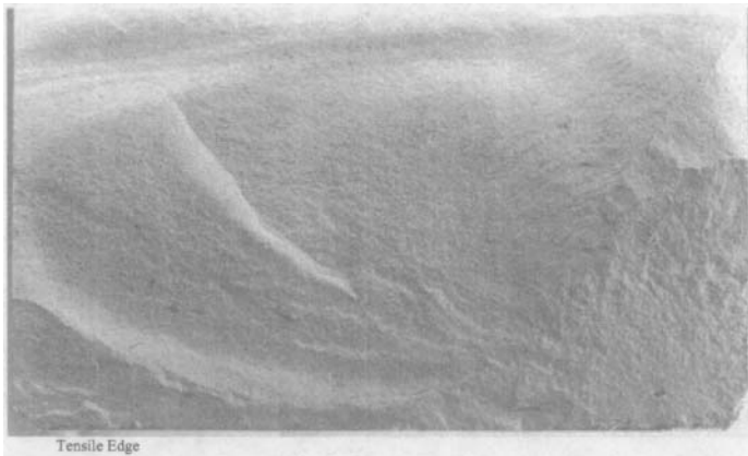
Figure 8. Bar II. Fracture Surface End Face – Composite [200x magnification]
