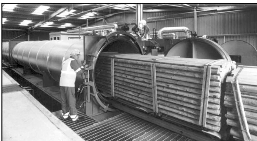
Plate 9 Vacuum-pressure impregnation treatment plant.
