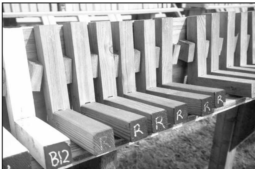
Plate 6 L-joint testing (EN 330) for coated and uncoated samples.
