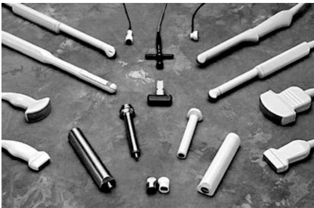
FIGURE 8.5 A photo showing several types of ultrasound probes including linear arrays and linear curved arrays, Doppler probes, and transrectal and transvaginal probes (long and slender ones in the upper half of the photo). (Courtesy of Sound Technology Inc., State College, Pennsylvania.)
