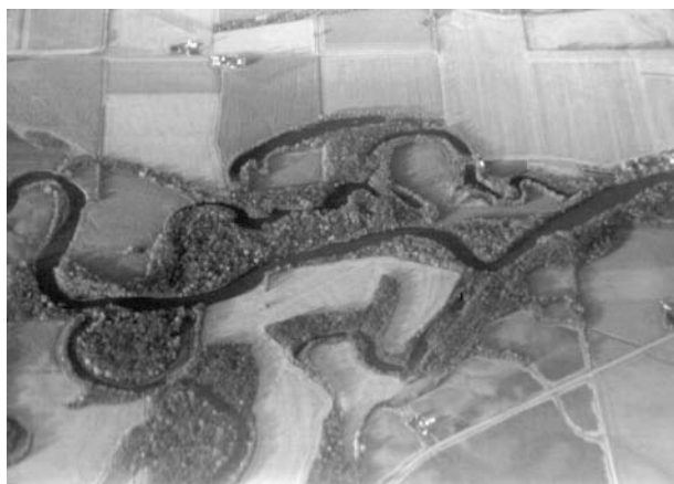
FIGURE 6.12 Formation of an oxbow at the bend in a stream. (Courtesy John Lyon.)
