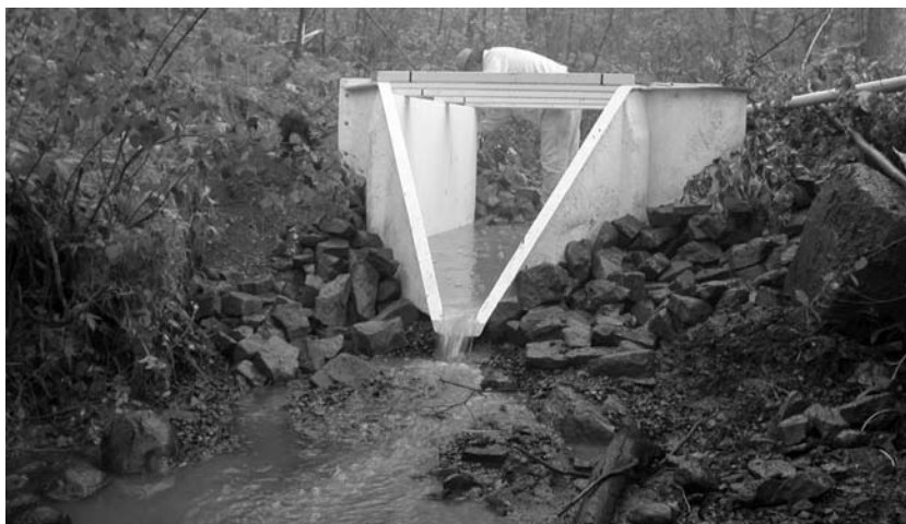
FIGURE 8.3 Flume in a stream. (Courtesy Kevin King.)
