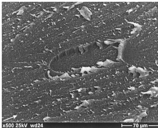
Figure 9. Epoxy/ \text{Al}_2\text{O}_3 nanocomposite containing 1 vol.% filler. Micro-rough structure, hyperbolic markings indicate the formation of secondary cracks. 19
