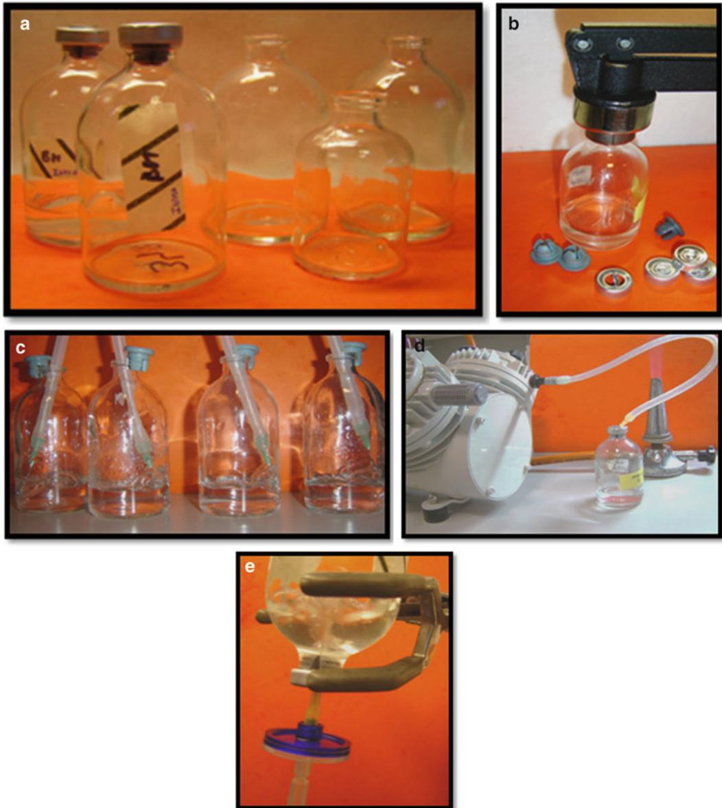
**Fig. 2** Bottles and tools used to prepare anaerobic cultures; bottles for culturing anoxygenic *R. rubrum*, chorobutyl rubber stoppers, and aluminum clamps (a) and hand crimper for crimping aluminum caps on vessels (b). Gas supply equipment. (c) Oxygen purging with nitrogen while putting the needle connected to the gas nozzle directly into the liquid. (d) Vacuum is done inside the bottle for 1 min prior to adding the syngas mixture. (e) The headspace of the vial is refilled with syngas
