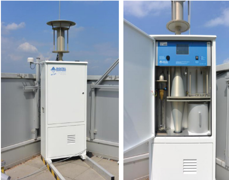
Figure 1.2.1 Digitel DHA-80 high-volume filter sampler operating from the roof of a building. (Photos: Anna Kunert, Max Planck Institute for Chemistry, Mainz, Germany.)
