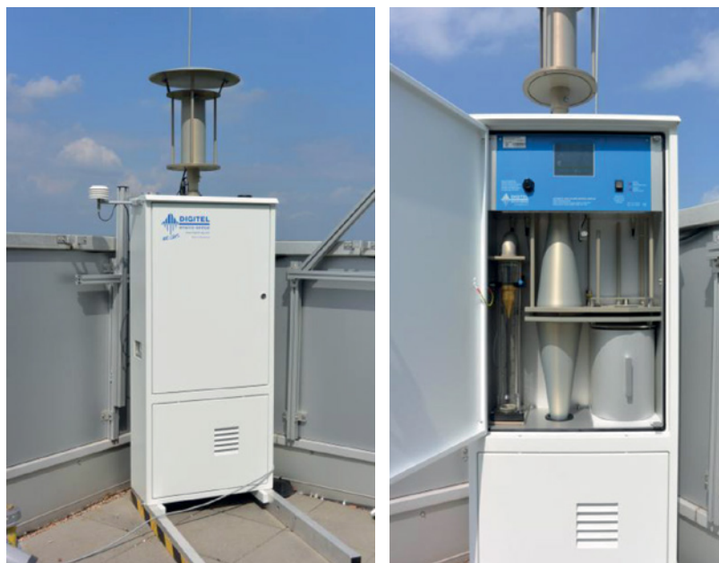
Figure 1.2.1 Digitel DHA-80 high-volume filter sampler operating from the roof of a building. (Photos: Anna Kunert, Max Planck Institute for Chemistry, Mainz, Germany.) (See color plate section for the color representation of this figure.)
