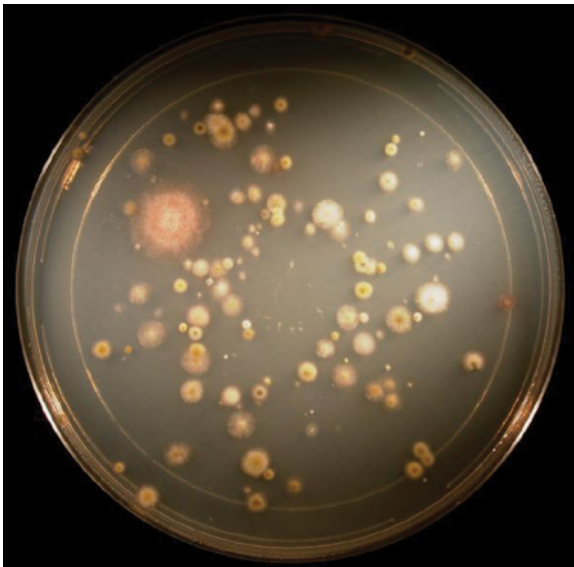
Figure 1.3.1 Colony-forming units on potato-dextrose-yeast extract agar (PDYA) medium from air sampled with a Casella CEL Airborne Bacteria Sampler (slit sampler). (Photo: T.C.J. Hill, Colorado State University, Colorado, USA.)
