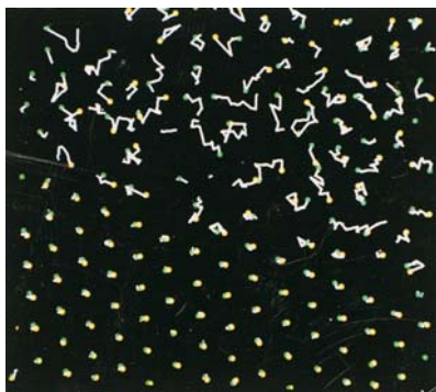
Fig. 4.12. Trajectory of particles in the two-state structure. Sample: polystyrene-based latex particle ( a = 150 nm, \sigma_a = 1.3 \mu\text{C cm}^{-2} ), \phi = 2 \times 10^{-2} , at rt. The particle centers in about 20 consecutive frames in 11/15 s are reproduced in a new frame and connected by straight lines. The particle positions at the starting time colored green and those after 11/15 s yellow. The upper half shows free particles whereas the lower half the ordered particles with the interparticle distance of about 1 \mu\text{m} . The white lines without either green or yellow ends or both indicate the out-of-plane movement of the particles. Taken from [17] with the permission of the American Chemical Society
