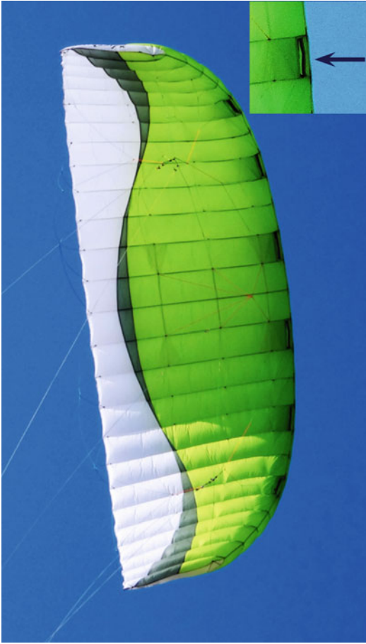
Fig. 15.1 Foil kite. Arrow shows one of the inlets through which the wind inflates the kite
