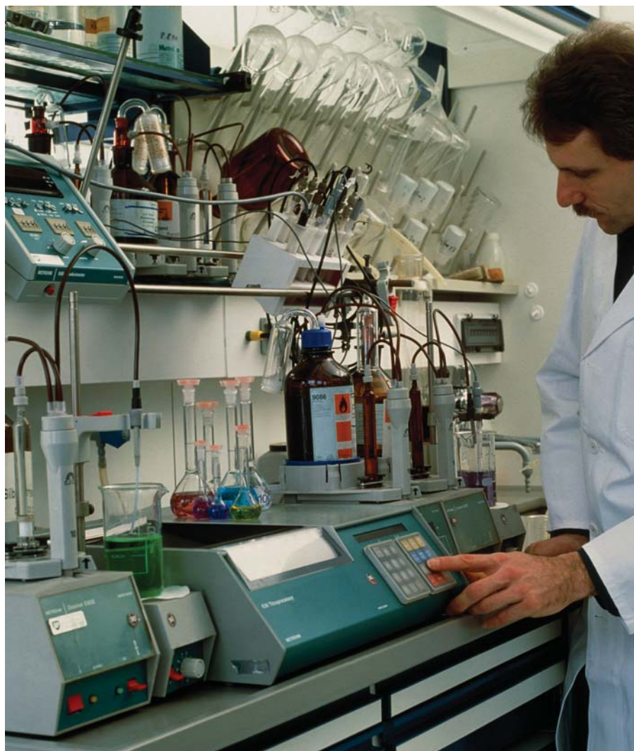
Figure 12.16 ▲ Chemist operating a computer controlled automatic titrator.
