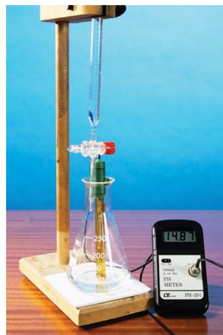
Figure 12.17 ▲ Apparatus for measuring the changes in pH during an acid–base titration.
