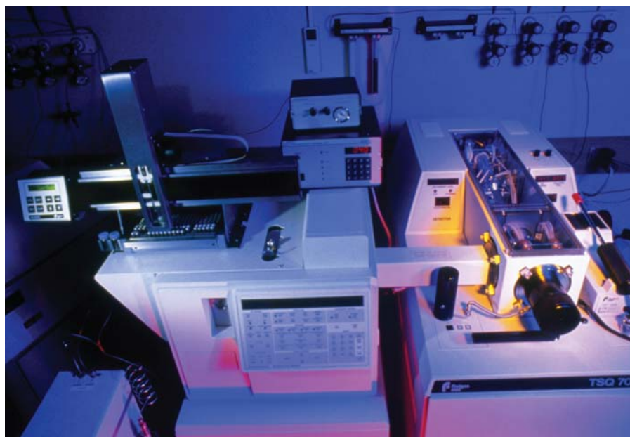
Figure 8.18 ▲ A gas chromatography machine (left) connected to a mass spectrometer (right) in a forensic laboratory. This equipment is sensitive enough to detect minute quantities of illegal drugs in the hair of a suspect – weeks after any drugs were taken.
