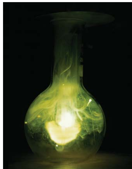
Figure 13.1▲ Hot sodium reacting with chlorine.
