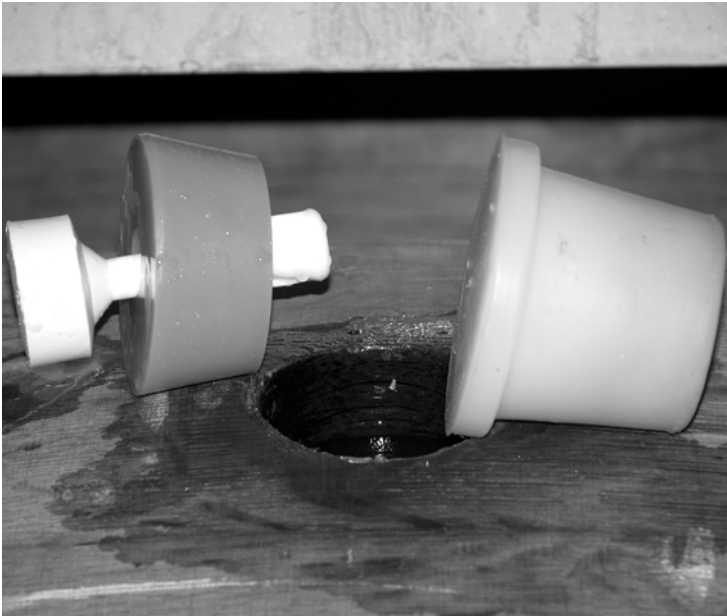
FIGURE 6.5. Barrel fermentation bung on the left and solid wine barrel bung on the right.
