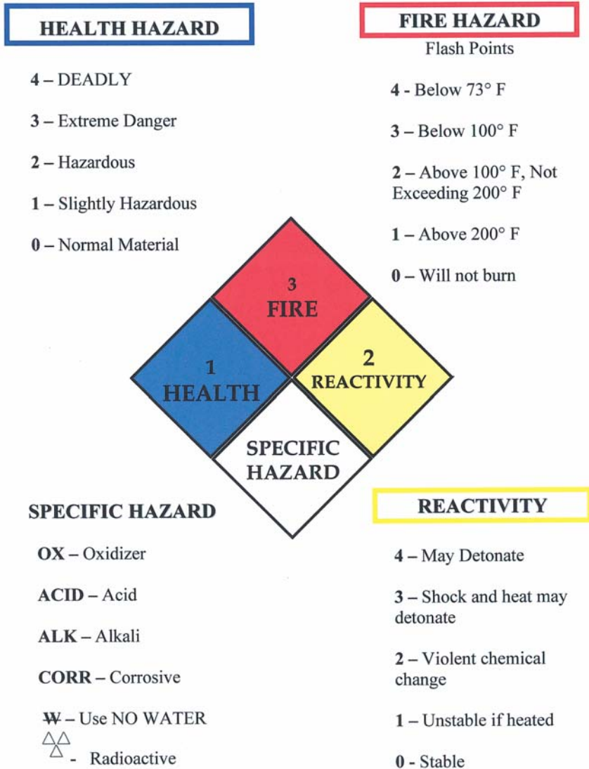
FIGURE 2.2. NFPA Hazard Classification (NFPA, 2001). This warning system is intended to be interpreted and applied only by properly trained individuals to identify fire, health, and stability hazards of chemicals. The user is referred to the recommended classifications of certain chemicals in the NFPA Guide to Hazardous Materials, which should be used as a guideline only. Whether the chemicals are classified by NFPA or not, those using the 704 system to classify chemicals does so at their own risk. (Reprinted with permission from NFPA 704-2001, System of Identification of Hazardous Materials for Emergency Response , Copyright © 2001, National Fire Protection Association, Quincy, MA.).
