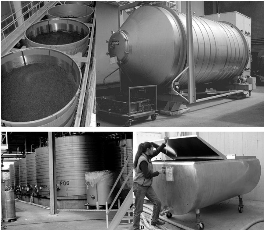
FIGURE 4.8. Red grape fermentation methods: (A) open top tank, (B) rotary fermentor, (C, D) tanks.
