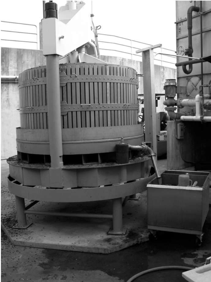
FIGURE 4.9. Typical basket press used to press the wine from the must.
