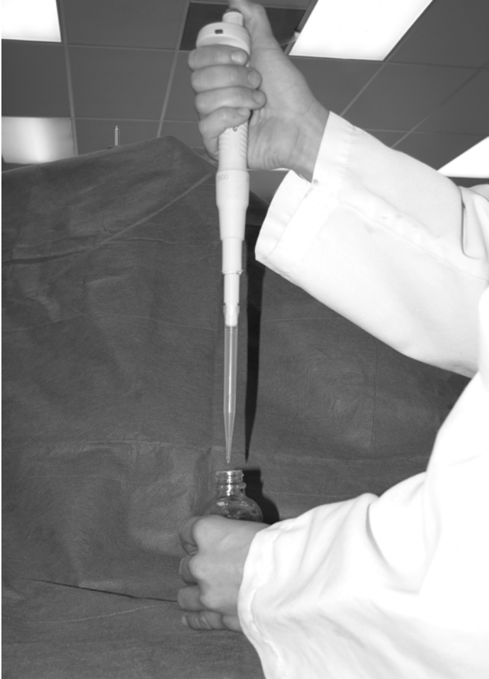
FIGURE 3.6. Correct automatic pipette position to aspirate liquid.
