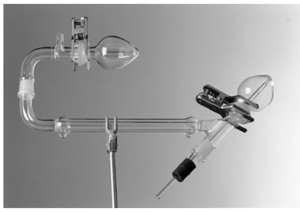
FIGURE 5.9. (A) Aeration-oxidation system for free, total, and bound SO 2 assays; (B) stopper with Pasteur pipette; (C) Graham condenser; (D) pear flask; (E) vacuum connecting tube with stem; (F) three-joint 90° (or 75°) tube; (G) stopper (not to scale). (B) Aeration-oxidation system for free SO 2 assay only: (A) round-bottom flask; (B) stopper with Pasteur pipette; (C) stoppers with glass connecting tubes; (D) pear flask; (E) vacuum connecting tube with stem (105° or 90° angle) (not to scale). (C) Research and Development Glass Products & Equipment's apparatus for SO 2 determination by aeration-oxidation.
