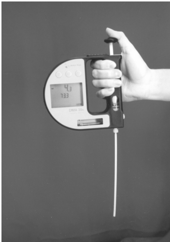
FIGURE 5.2. Anton Paar DMA 35n™ hand-held density meter with permanently stored concentration tables for °Brix, °Baumé, specific gravity, % alcohol, proof, °Plato, API gravity, and % H_2SO_4 . The units store 1000 data points and optionally downloads through an RS232 port.
