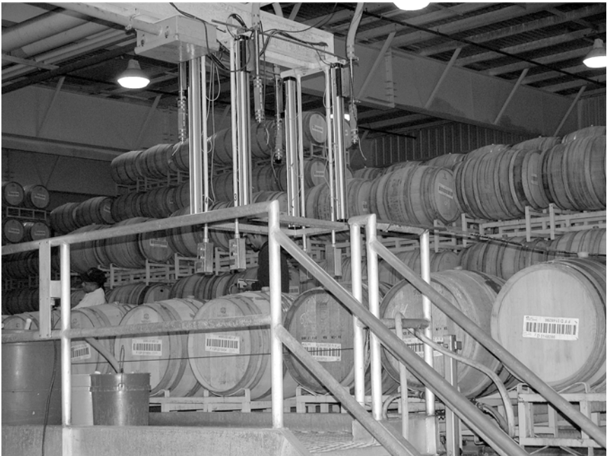
FIGURE 4.7. Manual and automated barrel filling.
