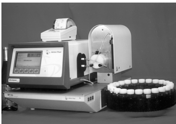
FIGURE 5.5. Anton Paar Alcolyzer ® NIR spectrometer for the determination of alcohol % v/v (based on ethanol tables). The Alcolyzer may be teamed up with the Anton Paar DMA 4500 ® or DMA 5000 ® density meter for determination of alcohol % w/w. The automatic sampler with bar-code reader holds up to 60 samples for attendant-free use.
