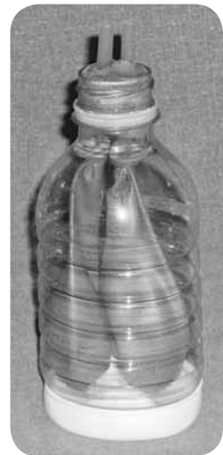
Figure 19.3 Balloon stretches over open bottom of bottle to create a diaphragm.
