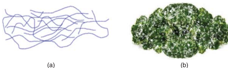
Figure 2.23 The structural shapes of acid and base catalyzed sol-gel reactions.
