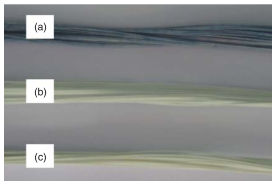
Figure 4.12 Comparison between the outer surface of control PES membrane and SPEEK-modified PES membrane after a chemical cleaning process, (a) control PES, (b) PES blended with 2 wt% SPEEK, and (c) PES blended with 4 wt% SPEEK. (Ismail 2009 [54]. Reproduced with permission of Taylor and Francis.)
