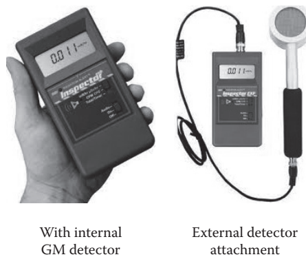
FIGURE 7.17 Analog and digital readout of GB-based detector systems.
