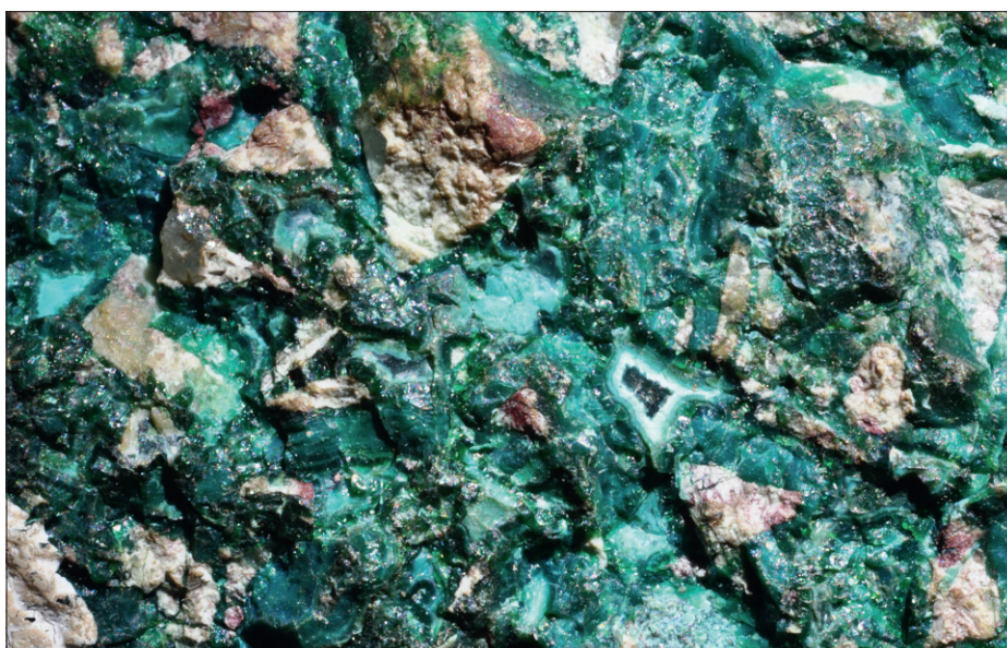
Fig. 8.35 Chrysocholla (Hydrated copper silicate). Colloform chrysocholla (blue-green) precipitating in cavities. Miami mine, Arizona, USA. Width of frame 5 cm.
