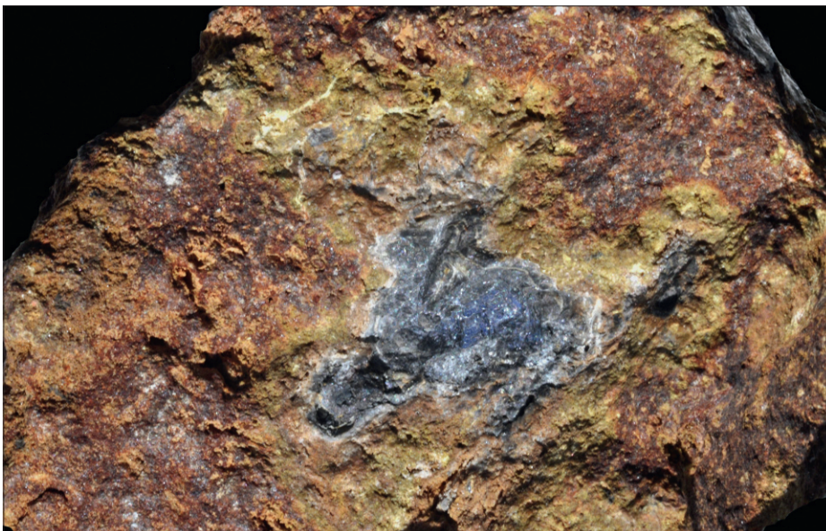
Fig. 6.38 Galena, anglesite, massicot and minium. Galena (dark grey – centre) surrounded by replacive cerussite (paler grey-glassy). The original cerussite layers (see Figures 6.37–6.38 ) are replaced by massicot (yellow) at near surface levels, and finally at surface the massicot is replaced by minium (red). Argentine district, Queensland, Australia. Width of frame 3.5 cm.
