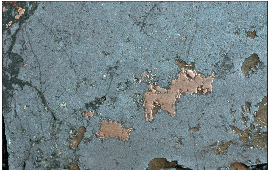
Fig. 6.10 Native copper. Infill cavity within grey metallic cuprite. Locality unknown. Width of frame 2 cm.
