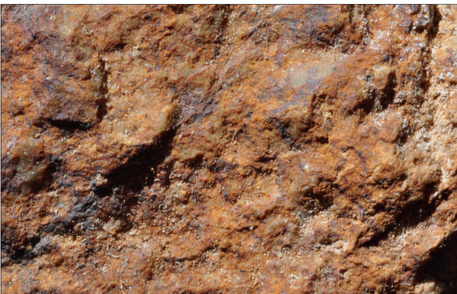
Fig. 8.24 Goethite dominant leached capping. Broken surface with abundant orange coloured transported limonite (goethite). Both this and adjacent disseminated styles would be assessed in terms of limonite styles and composition ( Table 8.1 and Figure 8.15 ). Original sulphide density would also be estimated –see text. Locality unknown. Width of frame 3 cm.
