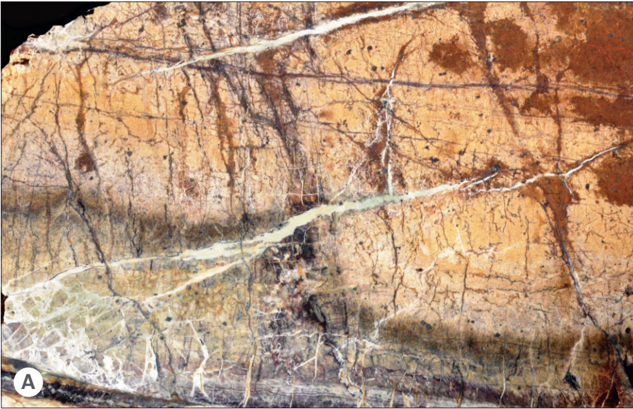
Fig. 7.46 False gossan – Serpentine. The three plates illustrate the progressive replacement of a leached serpentinite rock with prominent garnierite veining, to form a surficial limonite dominant replica. The final product is coarse celled, and in the field all stages of development are easily observed. The specimens come from 1 m depth (A) 4 cm depth (B) and the surface (C). Greenvale, Queensland, Australia. Width of frames 8 cm.
