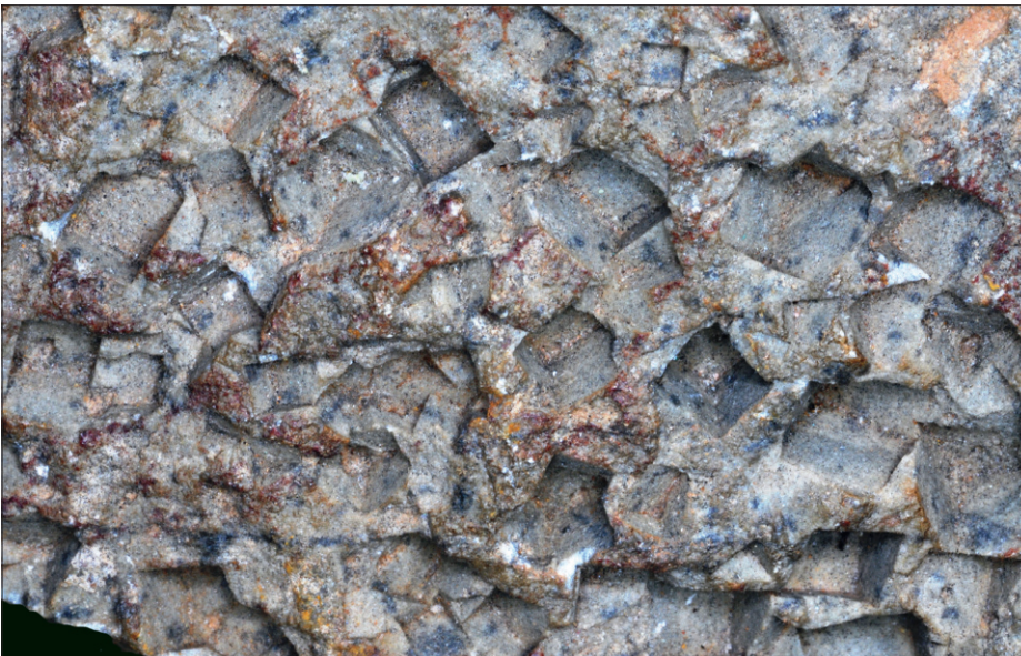
Fig. 7.3 Pyrite – negative pseudomorphs. Cube shaped cavities reflect the complete removal of pyrite. The low neutralising environment of a quartz-rich host rock discourages precipitation of indigenous limonite (see Figure 7.4 , below). Location unknown. Width of frame 4 cm.
