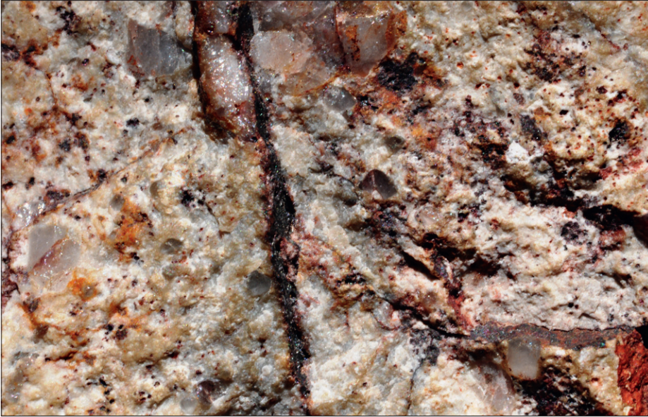
Fig. 8.22 Goethite dominant leached capping. Note the red-orange goethite colours in comparison with Figures 8.19–8.20 , showing the maroon colours of haematite dominant situations. The cavities are less full or even empty which coincides with an increase in transported limonite (see Table 8.1 ). The latter is showing up as precipitation along joints and fractures (bottom right hand corner and in tiny cracks (see also Figure 8.15 ). Location unknown. Width of frame 4.5 cm.
