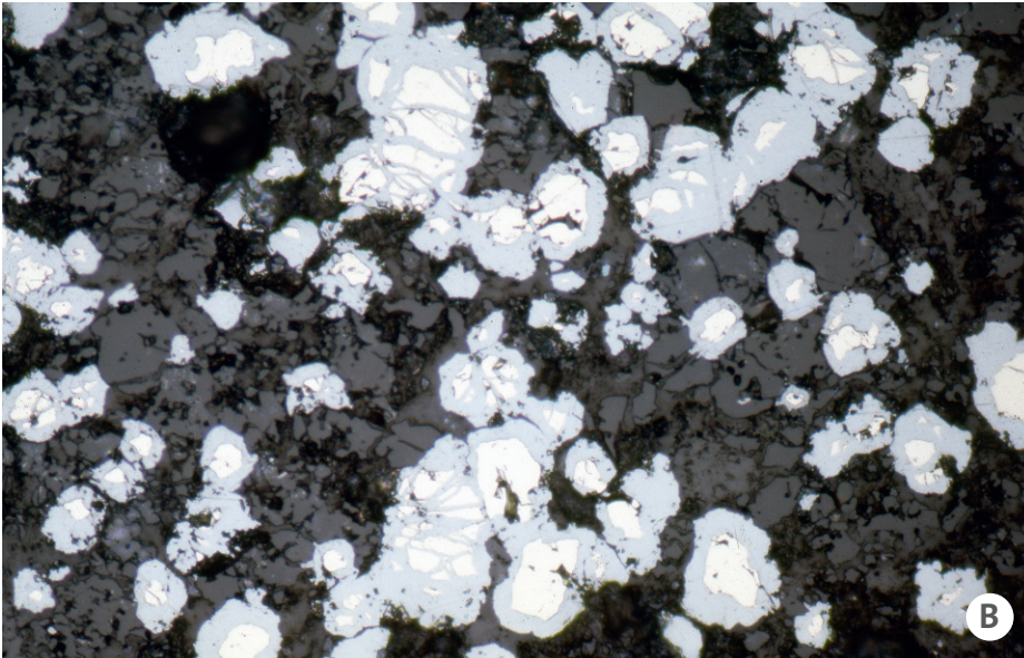
Fig. 8.12 B Supergene enrichment – polished sections. Advanced chalcocite development replacing pyrite. At this stage the profile would be referred to as mature. When replacement is minor the enrichment is called immature. Specimen from Escondida Norte, Chile. Width of frame 5.6 mm.
