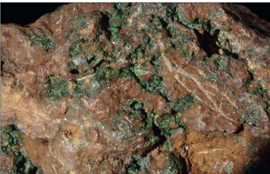
Fig. 6.56 Garnierite ("Nickel-magnesium hydrosilicate").
