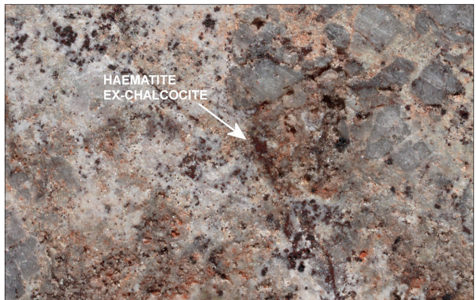
Fig. 8.44 Chalcocite spots (arrow) converted to haematite (indigenous). Minor transported haematite (see Figure 8.13). Host rock is breccia with quartz and porphyry fragments ± sulphide infill – alteration, sericite alteration and late clay overprint. Oxidised zone. DDH 118, 132 m. Width of frame 3 cm
