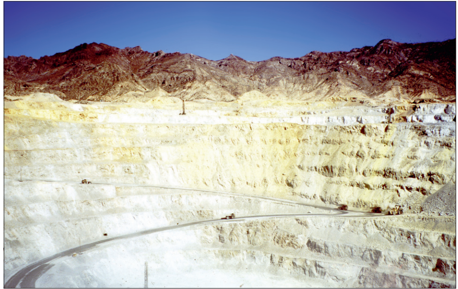
Fig. 8.10 Leached capping – jarositic ± minor goethite.
