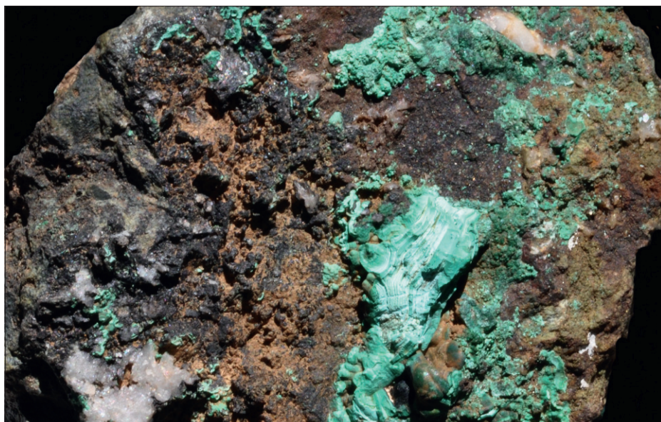
Fig. 8.38 Malachite (Copper carbonate). Botryoidal-colloform. Locality unknown. Width of frame 8 cm.
