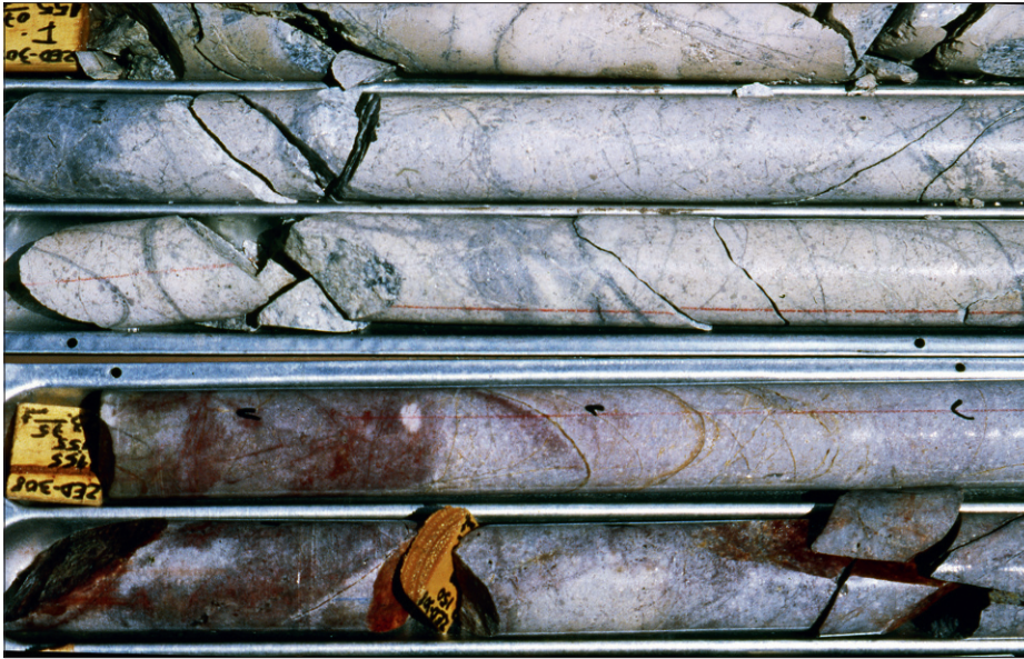
Fig. 8.16 Transition from chalcocite supergene enrichment zone (white-grey) to haematite altered oxide zone (red).
