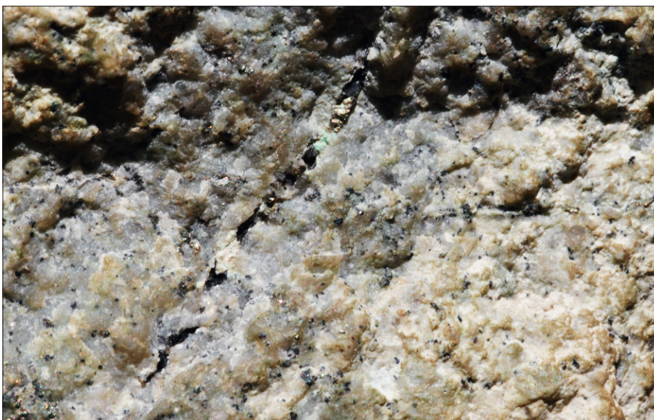
Fig. 8.18 Close up of an infill veinlet of quartz and sulphides (yellow and black) with an alteration halo of grey silica sericite (phyllic) alteration. The host rock is argillised porphyry. The dark sulphide is chalcocite forming as an alteration of chalcopyrite, and the yellow is unaltered pyrite (see Figure 8.12 A–B ). This is an example of incomplete supergene chalcocite alteration –sometimes referred to as immature.
