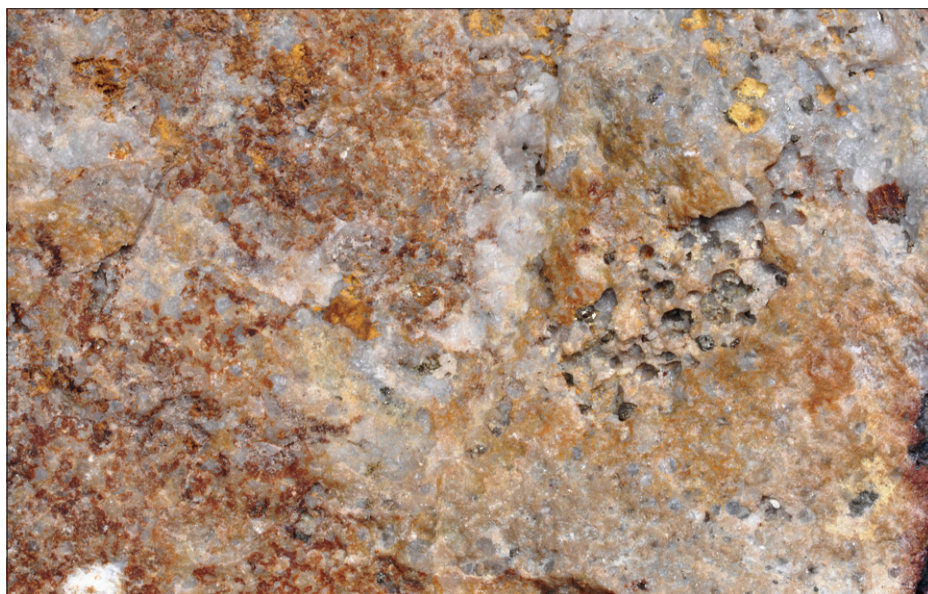
Fig. 7.6 Negative ovoid cellular pyrite pseudomorphs in a quartz vein, with remnant pyrite (see Figure 7.5 A). Home Hill district, Queensland, Australia. Width of frame 10 cm.
