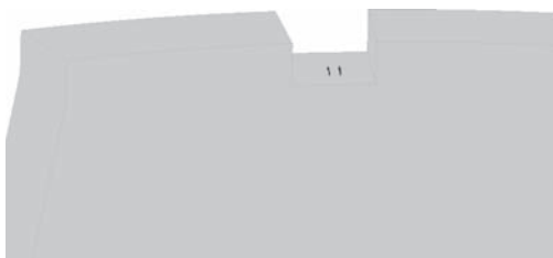
Figure 9. First crack location, between the shoes.
