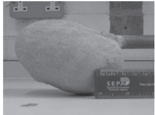
Figure 8. Hardened grout for w/c = 0.5 and b.c. = 4%.
