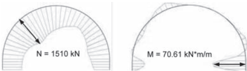
Figure 10. a) Axial force on primary lining; b) Bending moment.
