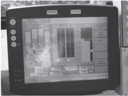
Figure 4. Rig operator's on-board computer screen.
