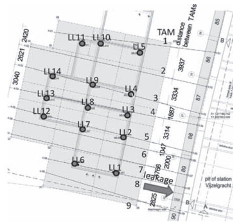
Figure 2. Top view of corrective grouting location, Vijzelgracht (distances between TAM's in mm).
