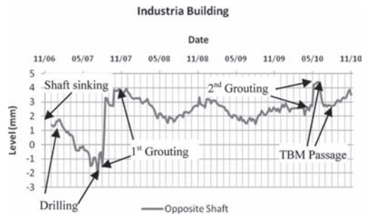
Figure 4. Monitoring of Industria building.
