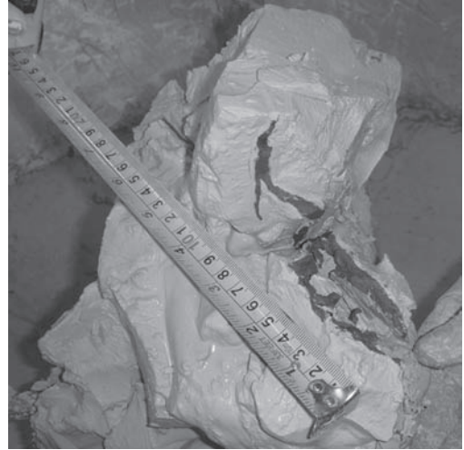
Figure 3. Grout injection in silt.
