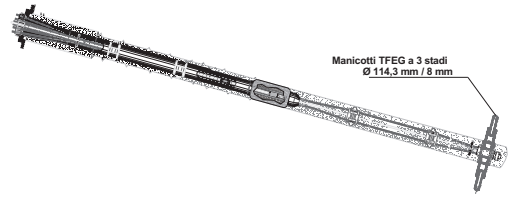
Figure 14. Tie-back equipped with TFEG.
