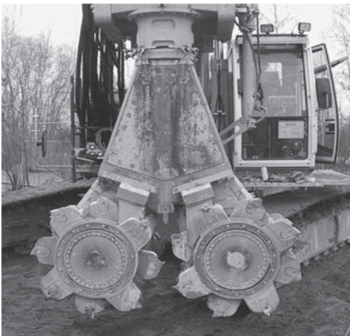
Figure 1. Mixing wheels and housing for hydraulic gear drives.
