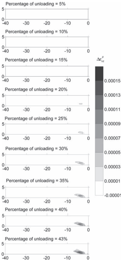
Figure 6. Increment in shear plastic strain in the masonry structure for different percentage of unloading.
