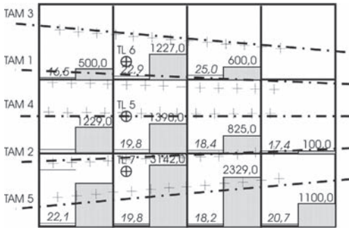
Figure 8. GroutControl plot of the area of the footing.
