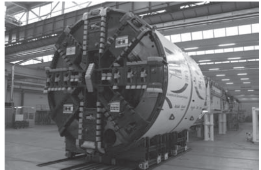
Figure 6. Photographs of the first EPB machine used for the excavation of the tunnels.
