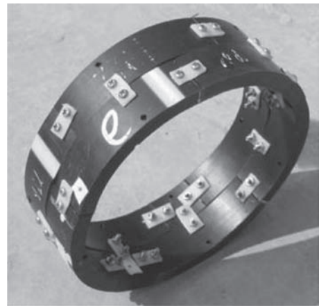
Figure 3. The assembly of the tunnel segments.
