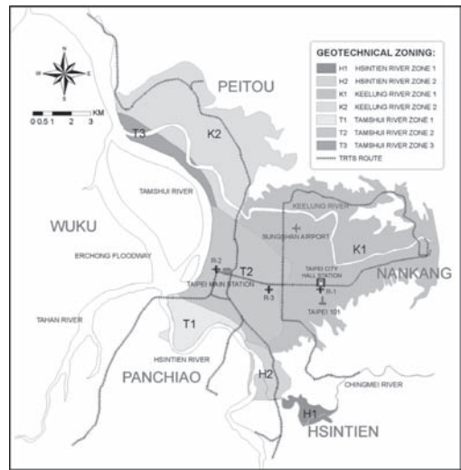
Figure 3. Geotechnical zoning of Taipei Basin with first stage network of TRTS (after Chin et al. 2006).
