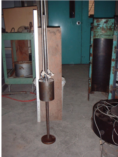
FIG. 2. View of the drop hammer used by Bray et al. (2009) for specimen preparation.
