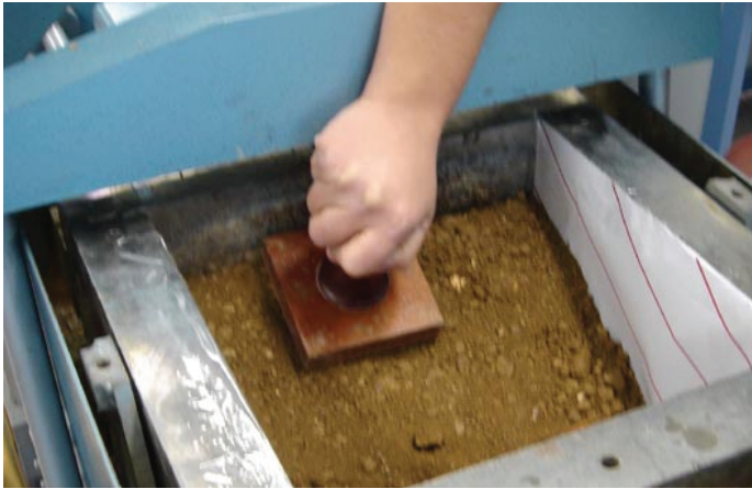
FIG. 4. A tamper being used for the preparation of synthetic waste direct shear specimen (from Athanasopoulos et al. 2008)
