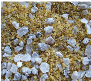
FIG.1. Leighton Buzzard:rock salt (80:20) mix.
