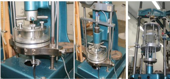
FIG. 5. Oedometric test with suction measurement and triaxial test with direct suction measurements. (after Izzo 2008)
