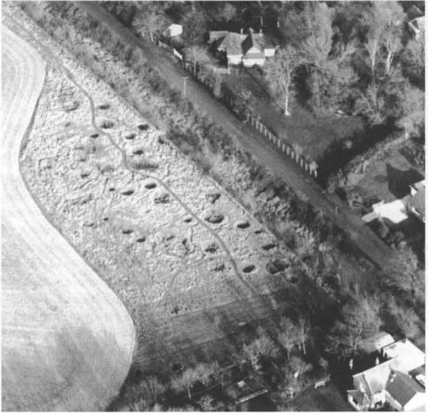
Fig. 3.1 Air photo showing extent of collapse features at Littleheath Road, West Sussex, UK (courtesy of Sealand Aerial Photography)
