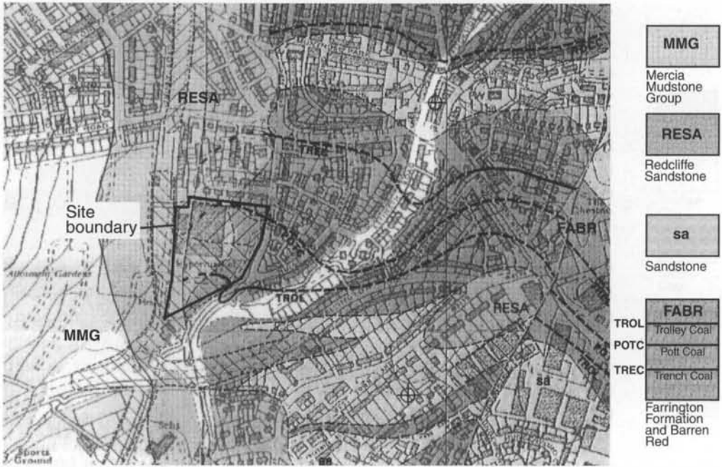
Fig. 2.5 1: 10 000 scale geological map – part of Sheet ST67 SW (Drift) of south-east Bristol (Reproduced with permission of BGS)
