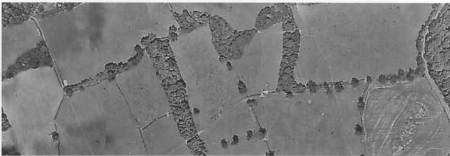
Fig. 2.14 Mosaic of vertical air photography, showing the landslip complex of the Sevenoaks by-pass site (after Clayton et al., 1995)
