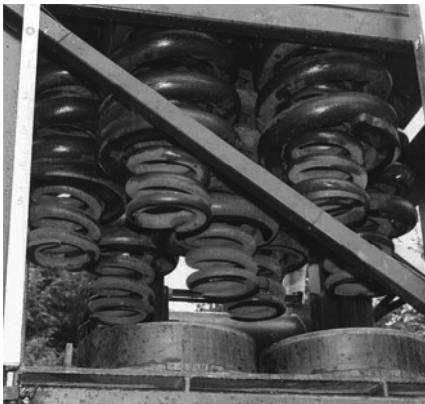
Figure 10.6 Example of a spring unit for extending force introduction
