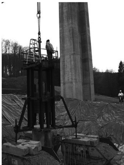
Figure 10.2 Loading system for cast-in-place concrete piles
