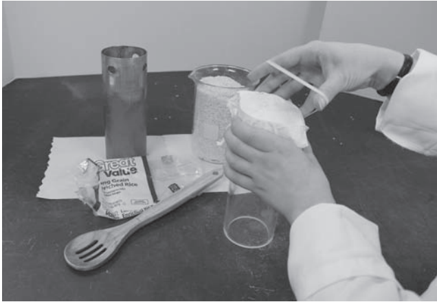
Figure 2-3. Attaching the paper towel to the tube
