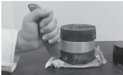
Figure 7-4. The demise of the potato chips; release of pore air pressure increases effective stress beyond the strength of the chips
