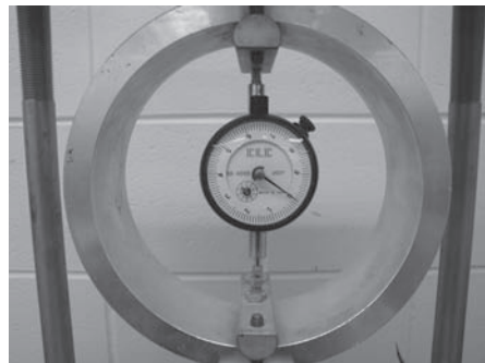
Figure 29-2. Left, sample in CBR apparatus, ready for testing; right, proving ring dial, used to calculate the force
