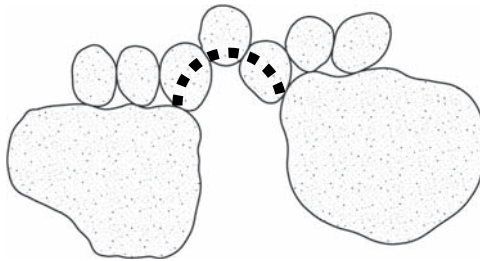
Figure 19-7. Arching schematic: the smaller soil particles above the larger ones do not fall through the larger space between the larger soil particles
