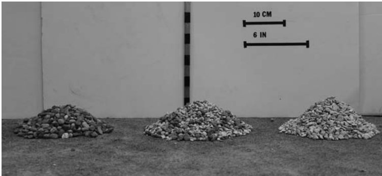
Figure 26-2. Three piles of gravel (left to right): rounded, subrounded, and angular; note the increasing slope angles
