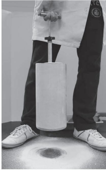
Figure 11-1. Lifting a cylinder of sand without direct connection between the cylinder and the lifting handle
