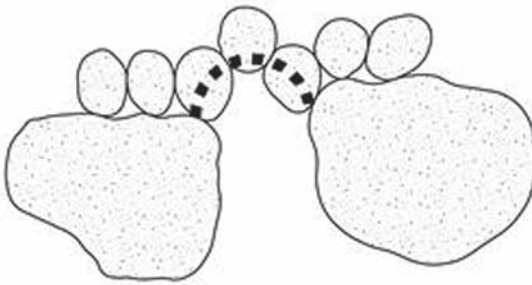
Figure 8-6. Two-dimensional arching schematic: the smaller soil particles above the larger ones do not fall down into the larger space between the larger soil particles; arch is shown by dashed line
