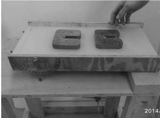
Figure 25-4. Top plate covering the soil, with weights in place
