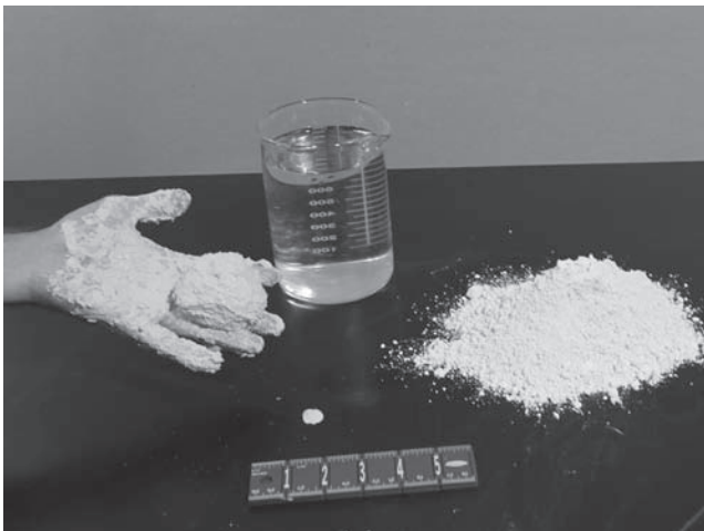
Figure 1-3. (R to L) Dry kaolinite, water, and wet kaolinite ball
