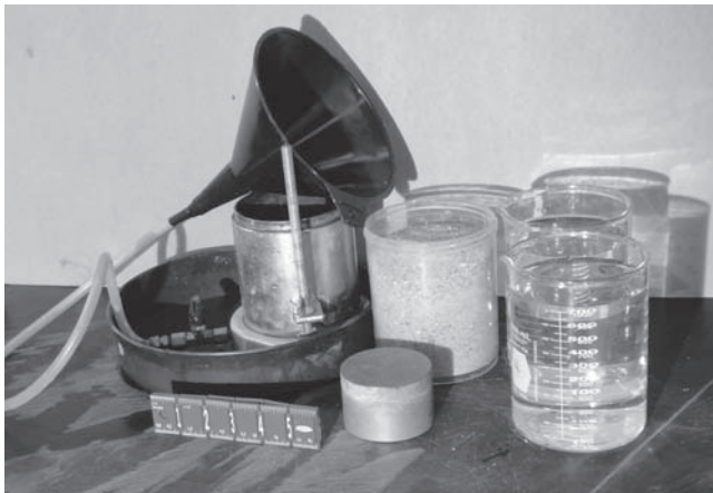
Figure 16-2. Funnel connected to permeability mold, weight, sand, and water; ring stand not shown; pan optional
