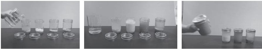
Figure 32-2. Left, adding water to the jars; center, jars awaiting caps; and right, capped jar being shaken
