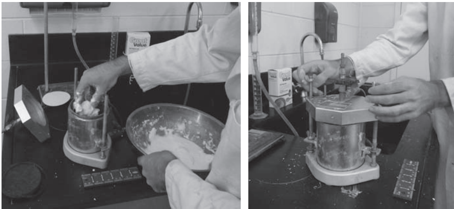
Figure 27-4. Placing oobleck in the falling head device (left) and assembling the falling head device (right)
