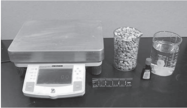
Figure 15-1. Balance, beaker of gravel, food coloring, and graduated beaker of water
