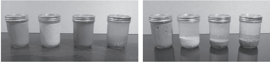
Figure 32-3. Left, jars immediately after shaking; right, jars two hours later, showing differential settlement
