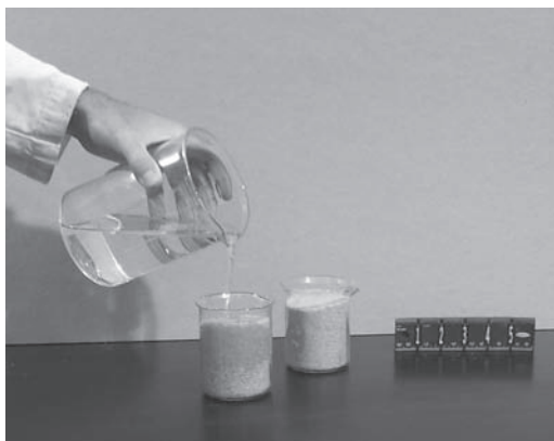
Figure 6-2. Left: adding dry sand to the beakers; right: adding water to one of the beakers
