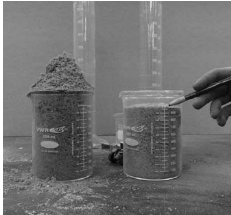
Figure 28-9. Comparison of replaced moist sand (left) and dry sand (right)
