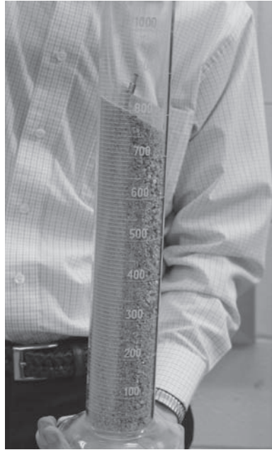
Figure 18-1. Graduated cylinder with dry sand in it (balance not shown)
