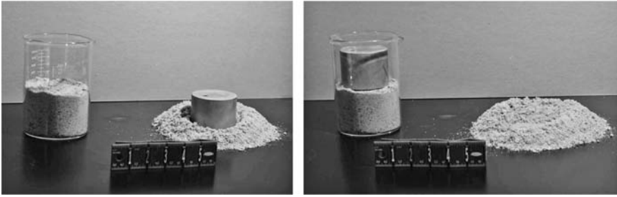
Figure 20-2. Left: weight crushing loose sand pile; right: weight having no effect on the confined sand in the jar
