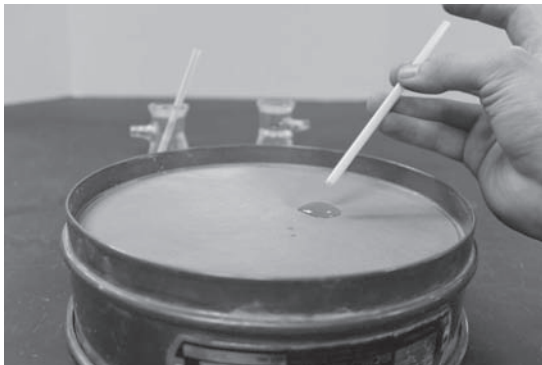
Figure 12-3. Water placed on the sieve forms a bead
