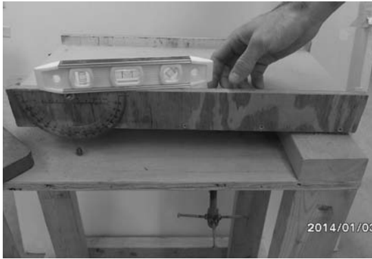
Figure 25-2. Leveling the sliding plane prior to operation; use the star wheel to adjust the table
