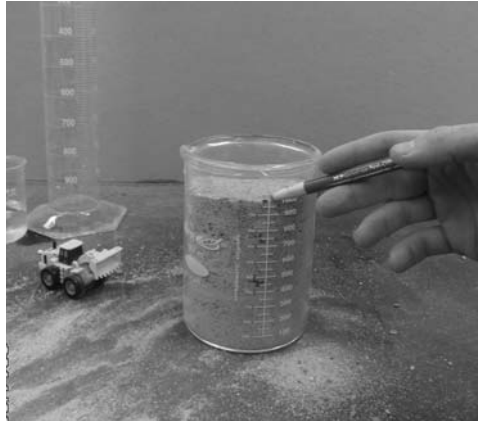
Figure 28-6. Replaced dry sand fills the beaker to the same level
