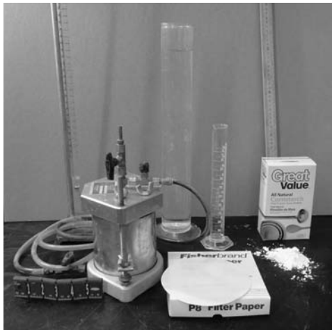
Figure 27-2. Standard hardware needed for the falling head test, plus corn starch
