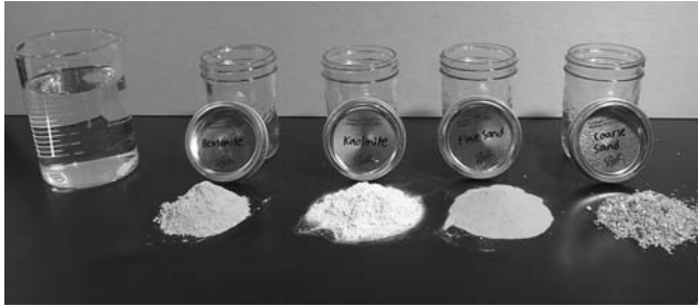
Figure 32-1. Water, four jars with four soil types (left to right): bentonite, kaolinite, silt, and coarse silty sand
