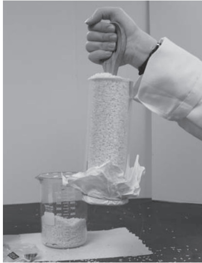
Figure 2-1. Tube of dry rice being held up by a spoon stuck in the rice
