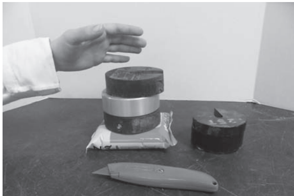
Figure 7-3. Placing weights on the bag of potato chips; note that the potato chips are still in the original, uncrushed, low effective stress condition
