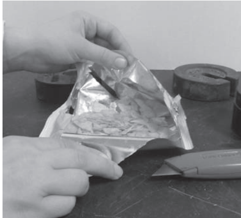
Figure 7-5. Crushed potato chips, after being subjected to high effective stress
