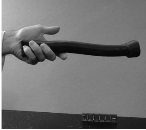
Figure 22-5. Tube with stoppers in both ends is now very stiff and strong
