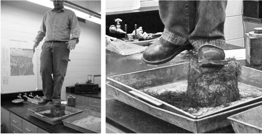
Figure 10-2. Left: person standing on Geofiber-reinforced sand (note non-Geofiber sand pile crushed on the right); right: close-up of Geofiber-reinforced sand with foot on it
