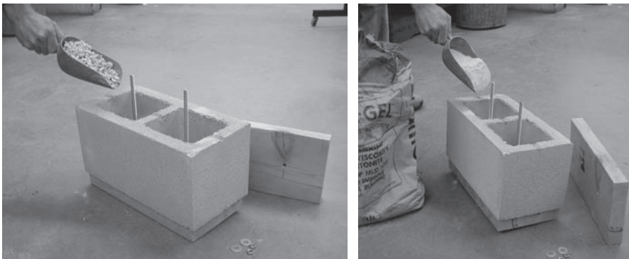
Figure 3-2. Left: assembled block, placement of the gravel layer; right: placement of bentonite over the gravel layer
