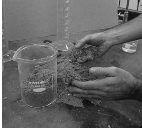
Figure 28-8. Replacing the moist sand in the beaker
