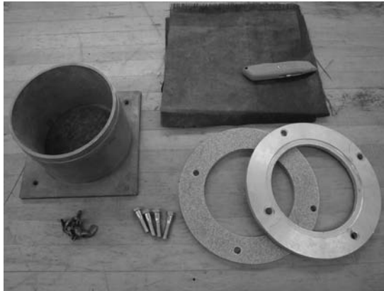
Figure 29-1. Geotextile puncture hardware: clockwise from lower right, two metal rings with holes, bolts, nuts, CBR mold, geotextile with utility knife; not shown: CBR piston and test frame
