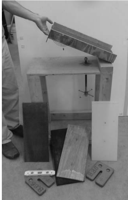
Figure 25-1. Tilt table device: from bottom, weights, level, and boards with varying frictional materials (note the star knob on threaded shaft for raising the table)
