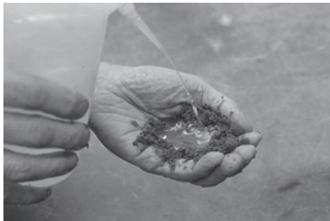
Figure 13-3. Saturating the silt
