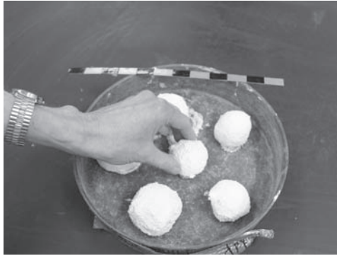
Figure 1-4. Wet kaolinite balls prepared for the oven
