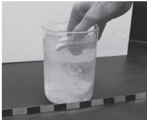
Figure 1-6. Dry ball, advanced slaking
