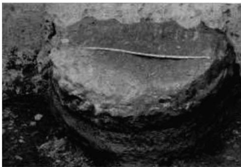
Figure 6.8 (a) Dual colliding jets. (b) Columns produced by dual colliding jets.
