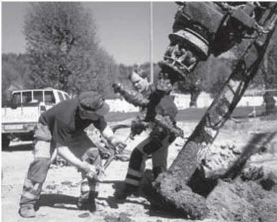
Figure 10.20 (a) Reverse column penetration test. (From Holmqvist, L. (1992). The lime column method. Bygg och Teknik , 7–8:40–44, in Swedish.) (b) Picture of installation of the probe. (Courtesy of LCM.)
