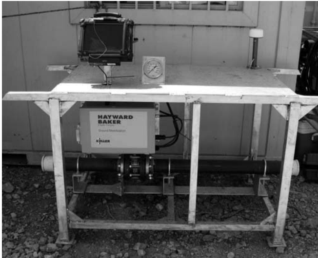
Figure 8.17 Compaction grout DAQ system with grout line under table where grout pressure and volume is measured. (Courtesy of Hayward Baker Inc.)
