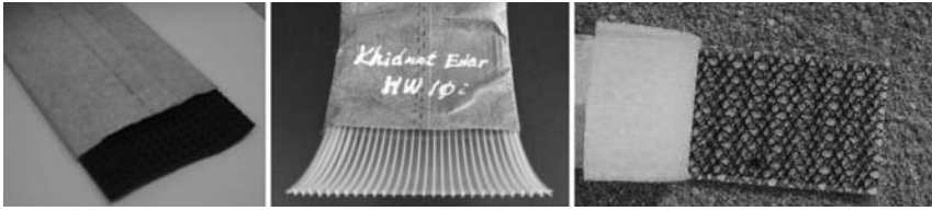
Figure 4.8 Samples of ordinary types of PVDs.
