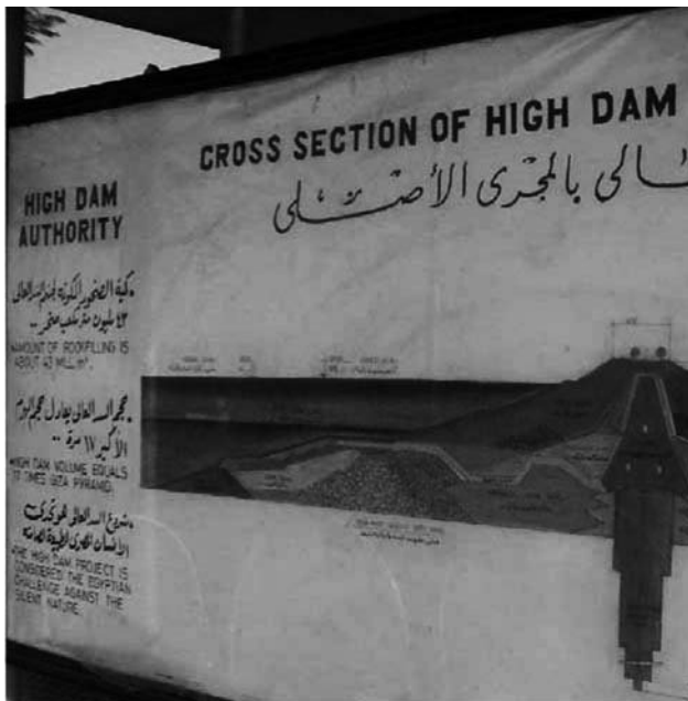
Figure 5.4 Recent view of a cross-section of Aswan High Dam (on-site tourist poster).
