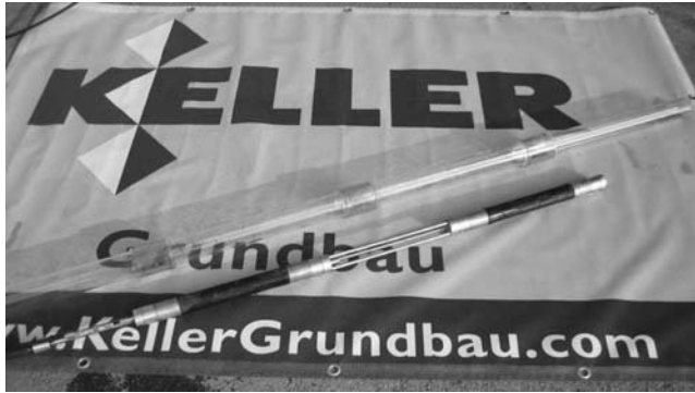
Figure 7.20 Double packer for 2" grouting pipes.
