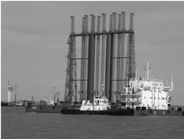
Figure 4.16 A PVD installation barge. (From Yan, S.W., Chu, J., Fan, Q.J., and Yan, Y. (2009). Building a breakwater with prefabricated caissons on soft clay. Proceedings of ICE, Geotechnical Engineering , Vol. 162, No. 1, pp. 3–12.)
