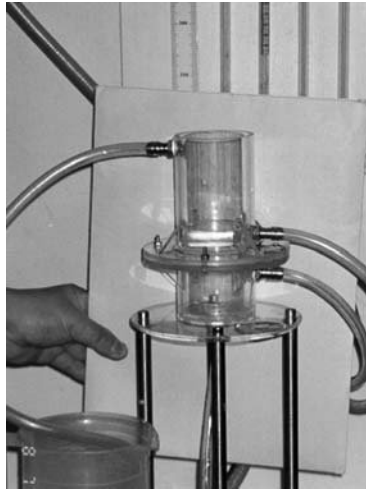
Figure 4.22 Device to measure the permeability of filter of PVD.
