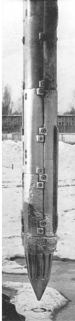
Figure 2.8 The Keller "Torpedo" vibrator
