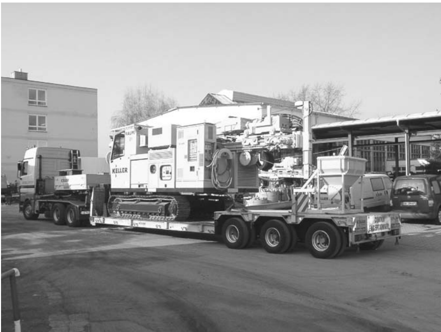
Figure 4.4 Minicat on low bed (by courtesy of Keller Group plc)
