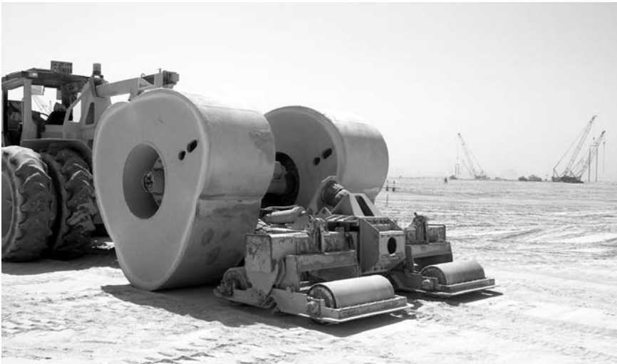
Figure 3.40 Impact roller in operation (by courtesy of Keller Group plc)
