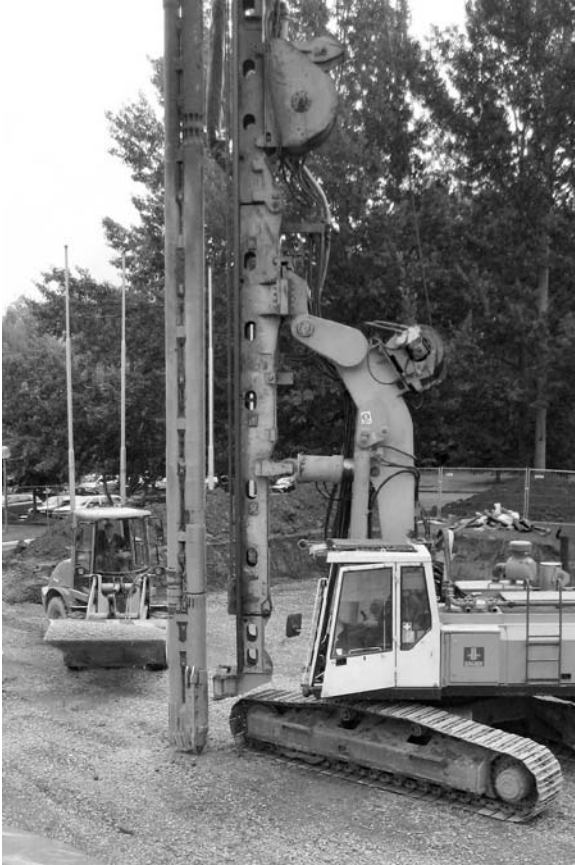
Figure 4.41 Bauer TR 17 bottom feed vibrator operated from BG12 base machine (by courtesy of Bauer)
