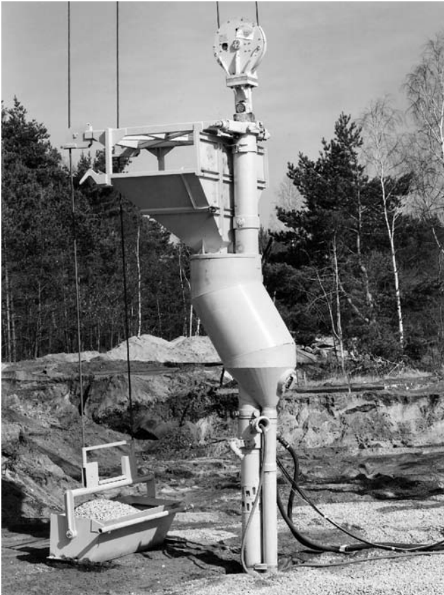
Figure 4.5 Crane-hung dry bottom feed system for deep stone columns (S-Alpha system) (by courtesy of Keller Group plc)
