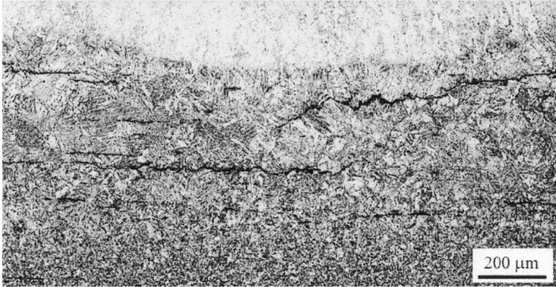
Figure 6-1: Hydrogen underbead (assisted) cracking in the HAZ of a single-pass, shielded-metal arc bead-on plate weld deposited on a C-Mn microalloy steel, from [28]
