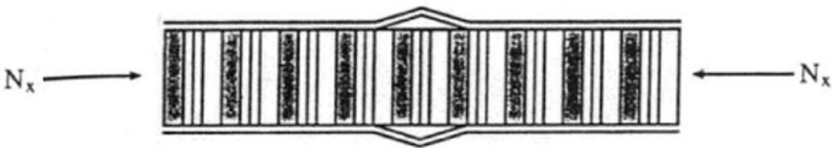
Figure 16.4. Face wrinkling instability. (Reprinted from References [1.7] and [10.1].)
