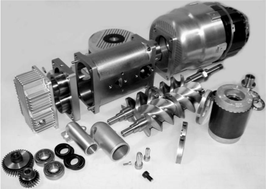
**Fig. 5.31.** Expanded View of the Compressor-Expander for Fuel Cell Application
