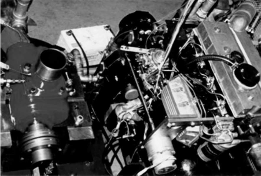
Fig. 4.8. 5-6-128 mm compressor in the air compressor test bed
