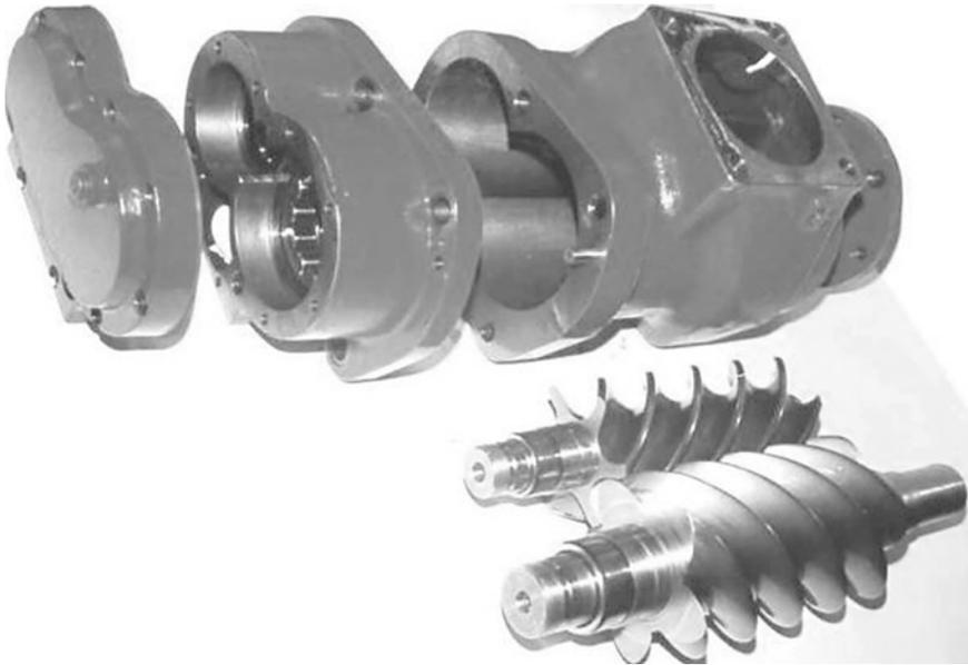
**Fig. 1.4.** Screw compressor mechanical parts
