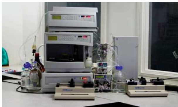
Fig. 7. Illustration of an automated reagent introduction, reaction and analysis set-up based on the incorporation of a micro-fluidic device into a conventional HPLC system
