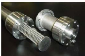
Fig. 16. a,b Two parallel microcapillary connection concepts: tube-and-shell multitubular and branched tube arrangements (Courtesy of ACS)
