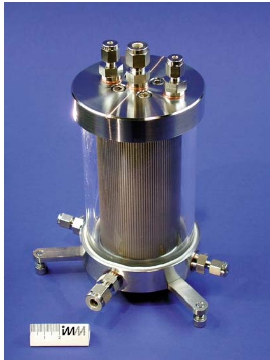
Fig. 12. Cylindrical falling film microreactor for pilot operation at tenfold capacity increase as compared to the laboratory falling film microreactor
