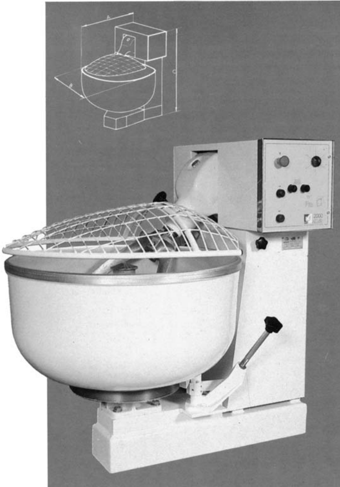
FIGURE 4.7. Oblique-axis or fork-type mixer (courtesy VMI).
