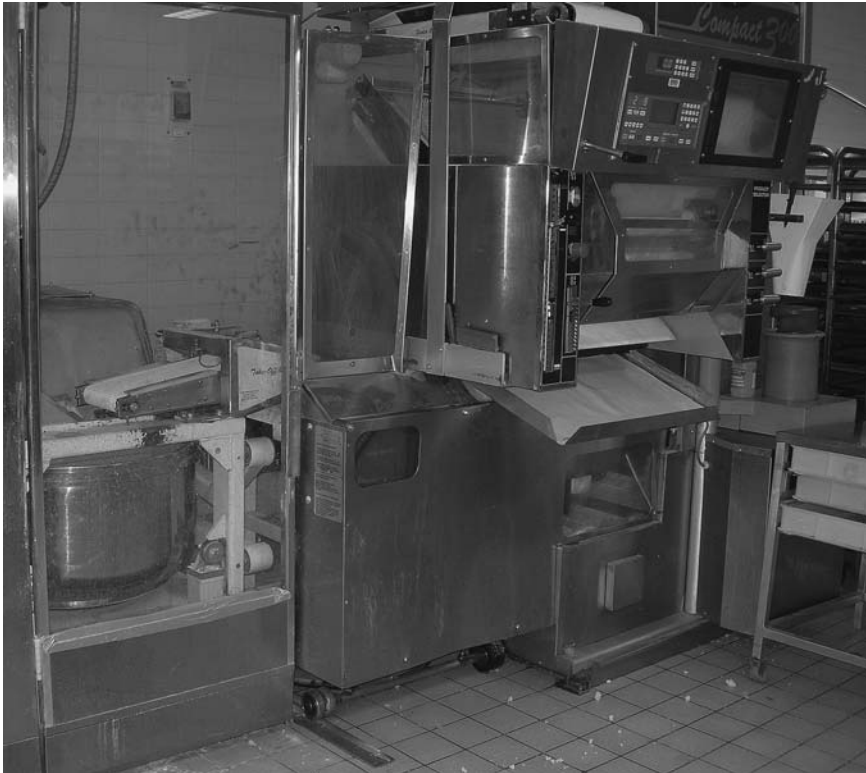
FIGURE 4.25. Combination bread and roll plant (courtesy J. Sainsbury).
