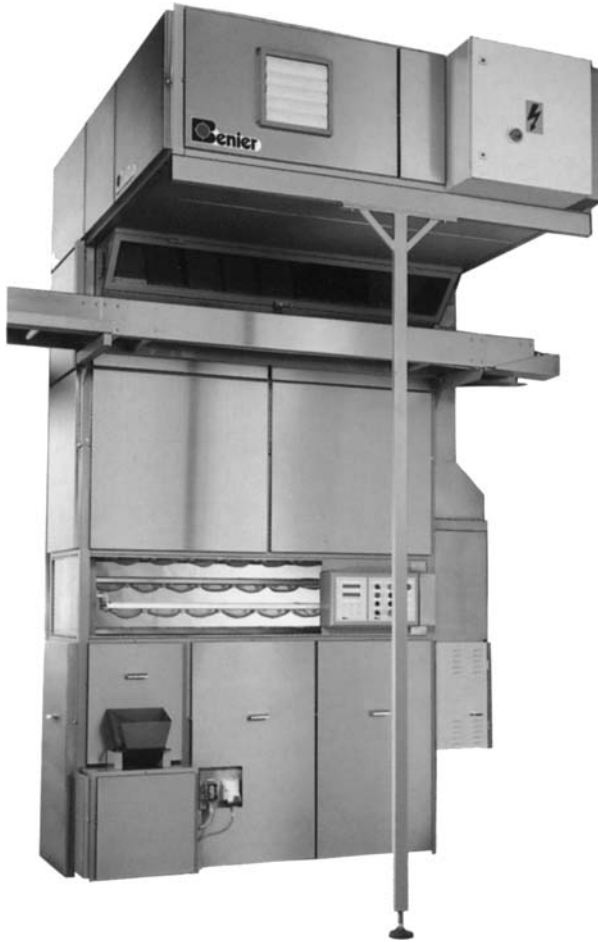
FIGURE 4.13. Pocket type first prover (courtesy Benier).
