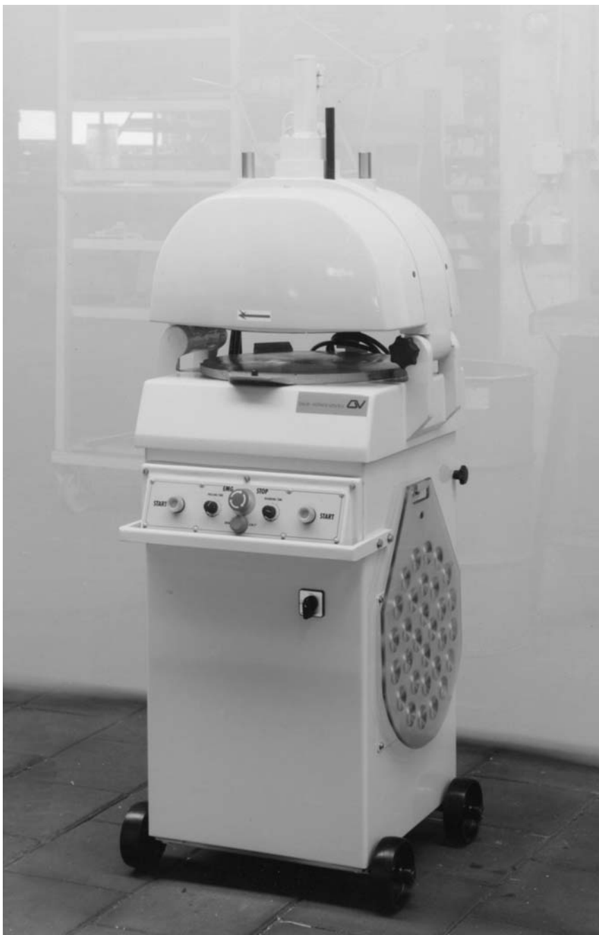
FIGURE 4.24. An automatic bun divider-moulder (courtesy Daub Verhoeven).
