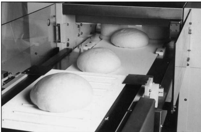
FIGURE 4.18. Dough piece being centred before sheeting.
