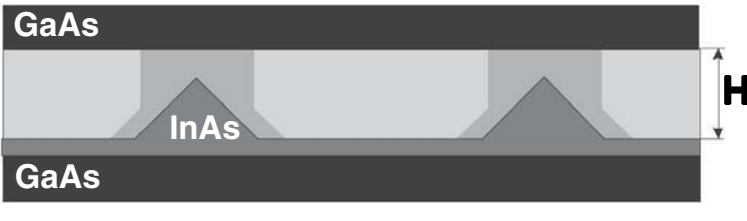
Figure 1. Schematic diagram illustrating activated alloy phase separation. (a) Initial InAs stressors, (b) partial decomposition of the alloy layer due to strain-driven surface migration of Indium, and (c) the final structure after GaAs capping.
